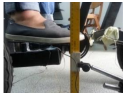
The height of the rear axle with a load of 77 kg is 190 mm
