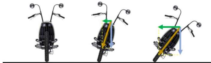
Fig. 3.5 - The lateral tilt of a motorcycle to counteract the centrifugal force. [19] (green - centrifugal force, blue - gravitational force, yellow - resultant force)
