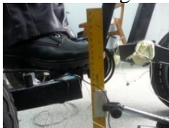
The height of the rear axle with a load of 44 kg is 204 mm
