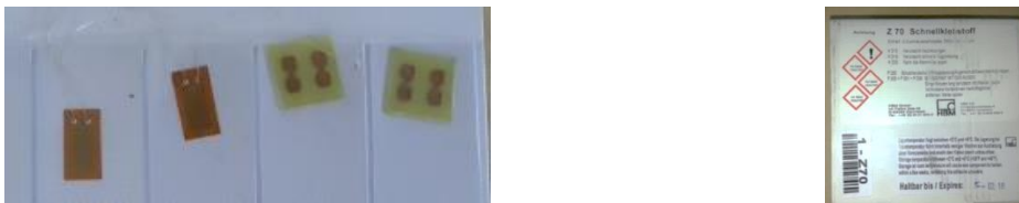
Fig. 6.3 - Tensometric transducers and the adhesive used
