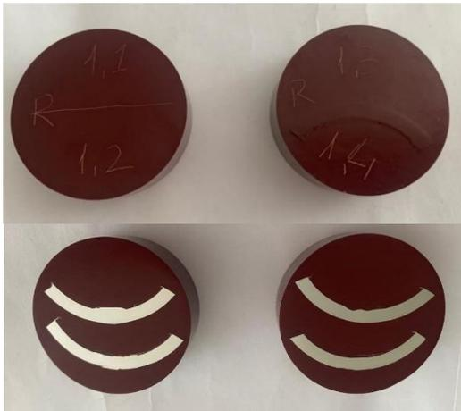
**Figure 6.8.** Sample 1 – positioning of welding points [33], 1.1. – point 1 - 50 mm; 1.2 – point 2 - 100m; 1.3. – point 3 - 150 mm; 1.4 - point 4 - 200 mm [33]
