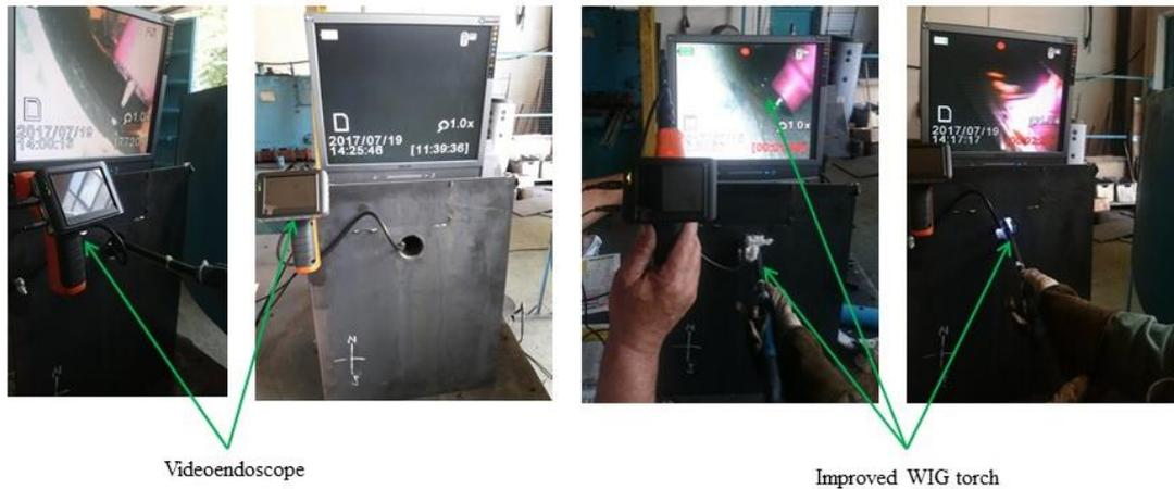
**Figure 4.2.** Experimental welding equipment built [29]
