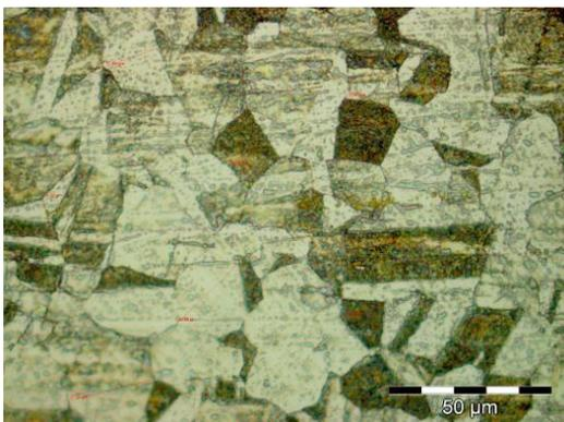
**Figure. 6.10.** Parent material microstructure
