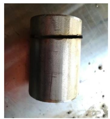
**Figure 5.3.** Austenitic stainless steel pipe X2CrNiMo17-12-2, sample 5 [31]
