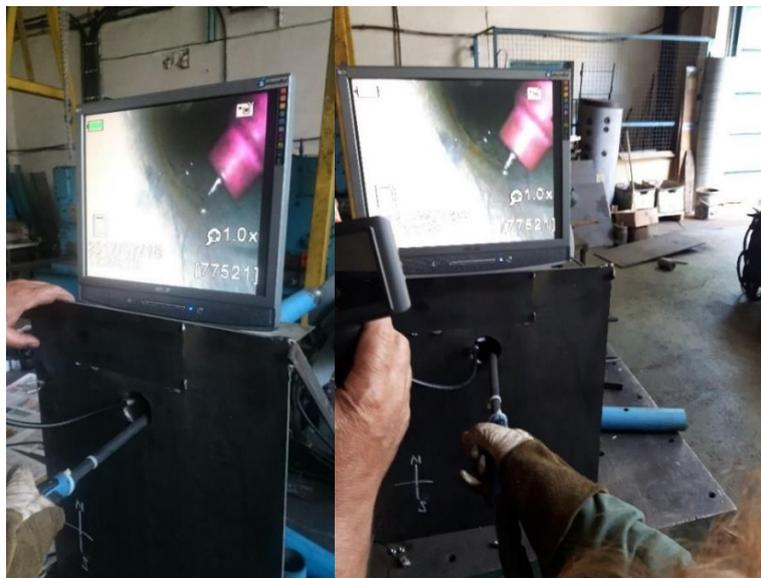
**Figure 5.4.** Welding repair of samples [31, 33]
