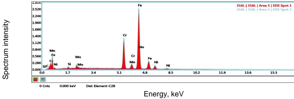
Figure 6.20. Parent material chemical elements distribution spectrum determined by EDAX analysis
