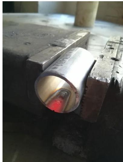
**Figure 5.9.** Sample 4 – linear defect along the length of the pipe
