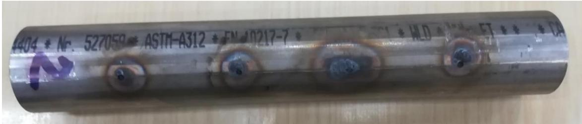
**Figure 5.6.** Sample 2 – 3 mm diameter holes
