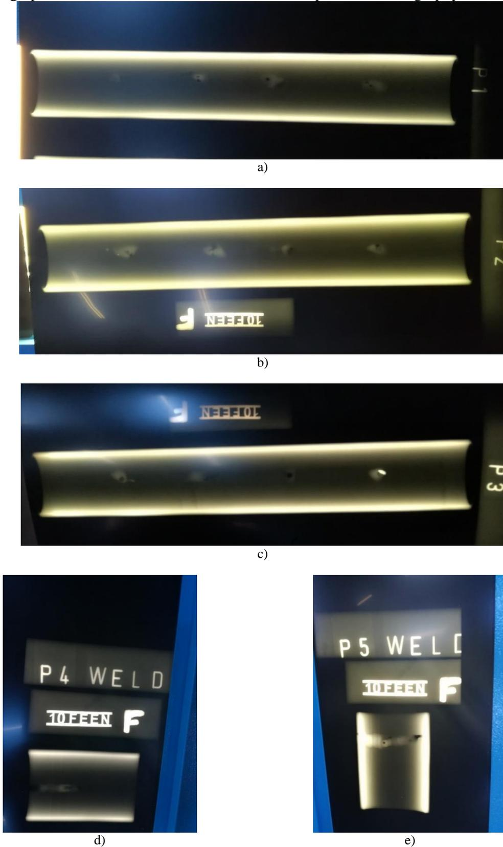
**Figure 6.7.** Images obtained after penetrant radiography.
