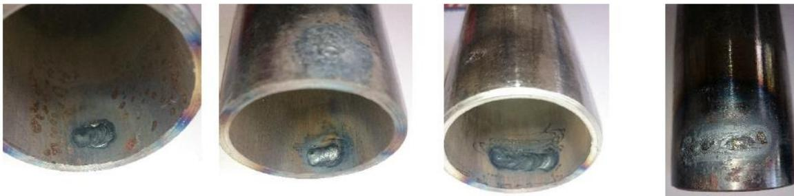
Figure 4. 6. Pipe type samples repaired by welding
