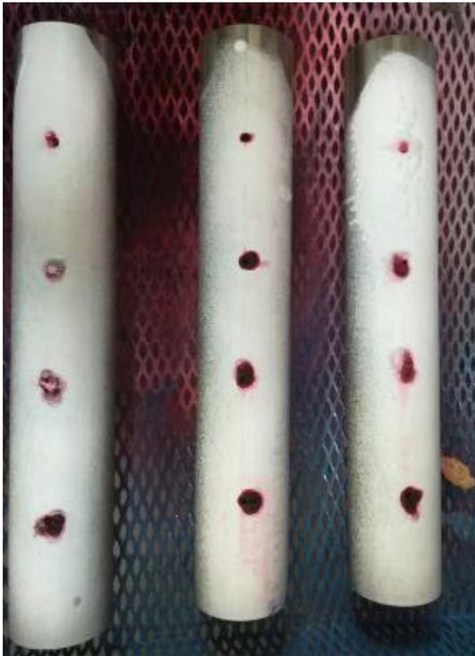
**Figure 6.5.** Developer application samples 1÷3
