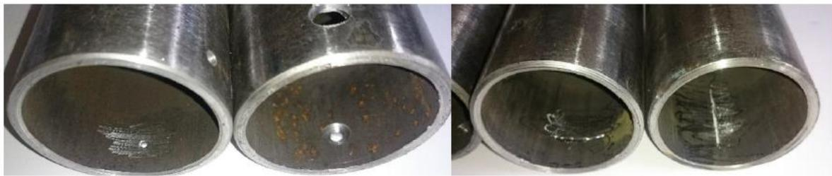
Figure 4. 5. Pipe-type products with artificially created defects
