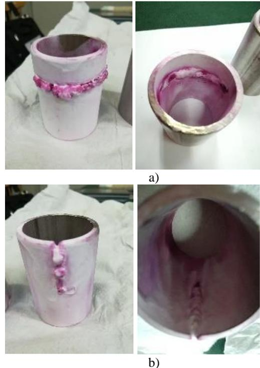
**Figure 6.6.** Developer application, a) inner and outer of sample 4, b) inner and outer of sample 5
