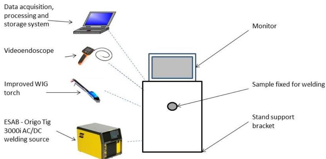
**Figure 4.1.** Experimental welding equipment diagram [32]
