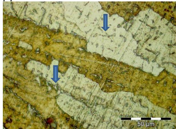
**Figure 6.17.** Welding root (1000x)
