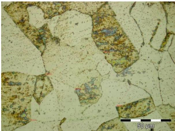
**Figure 6.13.** HAZ – overheating area with coarse polyhedral grains (500x)
