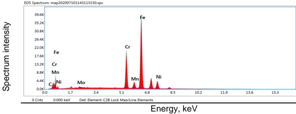
Figure 6.22. Parent material chemical elements distribution spectrum determined by EDAX analysis
