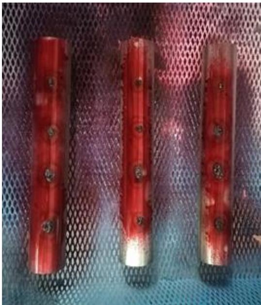
**Figure 6.3.** Penetrant application - samples 1÷3
