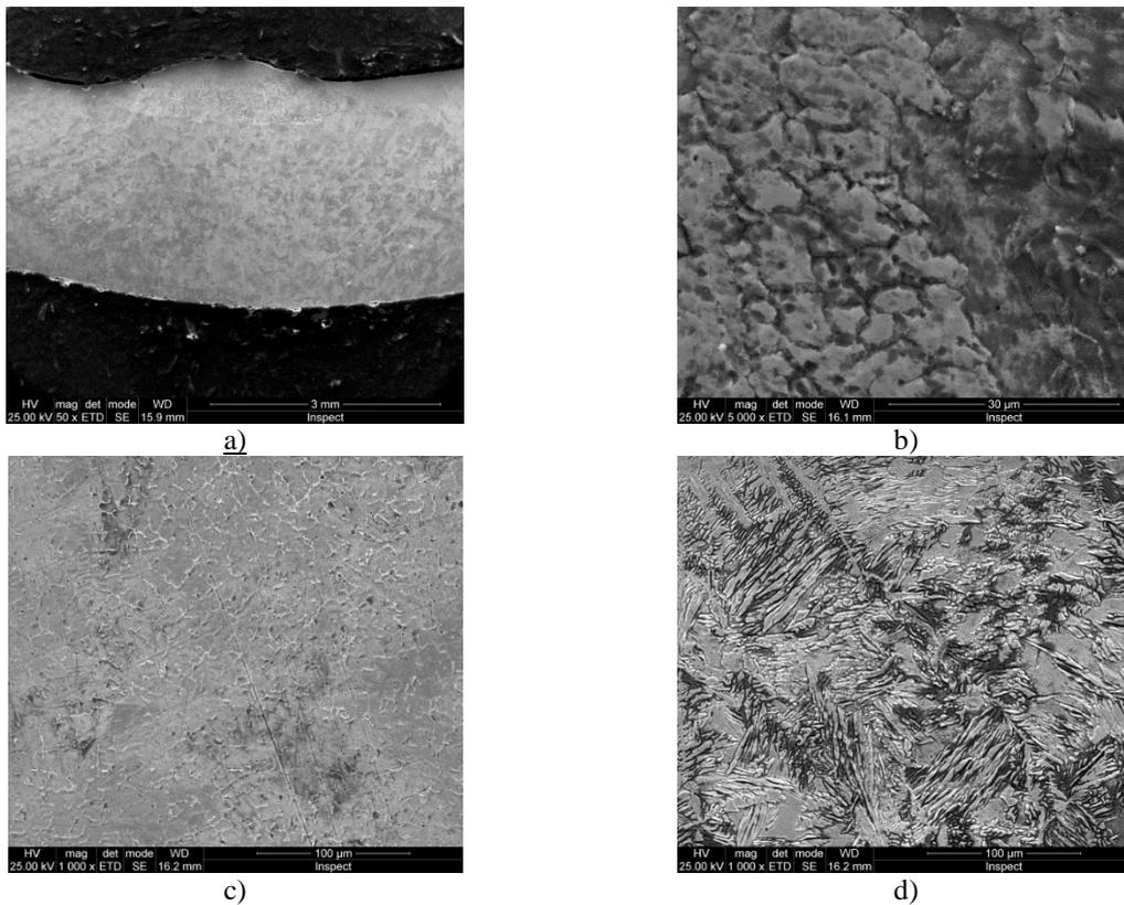
Figure 6.21. Micrographic images from different areas of the welded seam, a) Welding (50x), macroscopic appearance of the welded joint, b) Welding (5000x) Austenite - dendritic microstructure and fine films of intergranular delta ferrite, c) Fine austenite microstructure with dendritic appearance, d) Welding (5000x) Austenite, ferrite and martensite.
