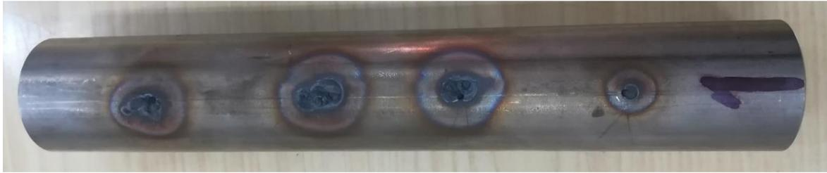
**Figure 5.5.** Sample 1 – 2 mm diameter holes
