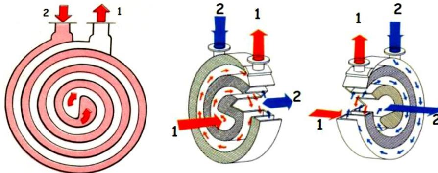
**Figure 1.2.** Working principle of a spiral heat exchanger [43]
