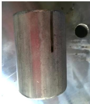
**Figure 5.2.** Austenitic stainless steel pipe X2CrNiMo17-12-2, sample 4 [31]
