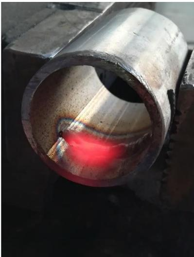
**Figure 5.8.** Sample 5 – linear defect on the circumference
