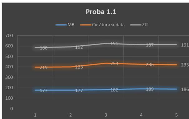
Figure 6.24. Hardness values graph for sample 1.1 [32]
