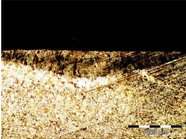
**Figure. 6.11.** Welding cross section (50x)
