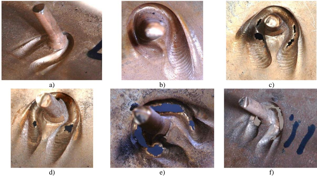
**Figure 2.1.** Defects that appeared due to the cavitation and corrosion phenomena [30]
