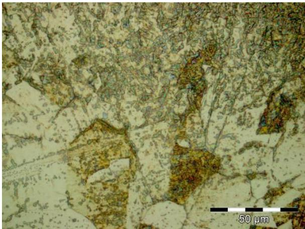
**Figure 6.12.** Parent material dilution area (500x)
