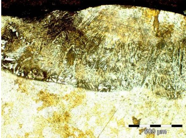
**Figure 6.14.** Welding final layer (100x)
