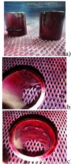
**Figure 6.4.** Penetrant application – sample 4 and 5, a) outer of the samples 4 and 5, b), c) inner of the samples 4 and 5
