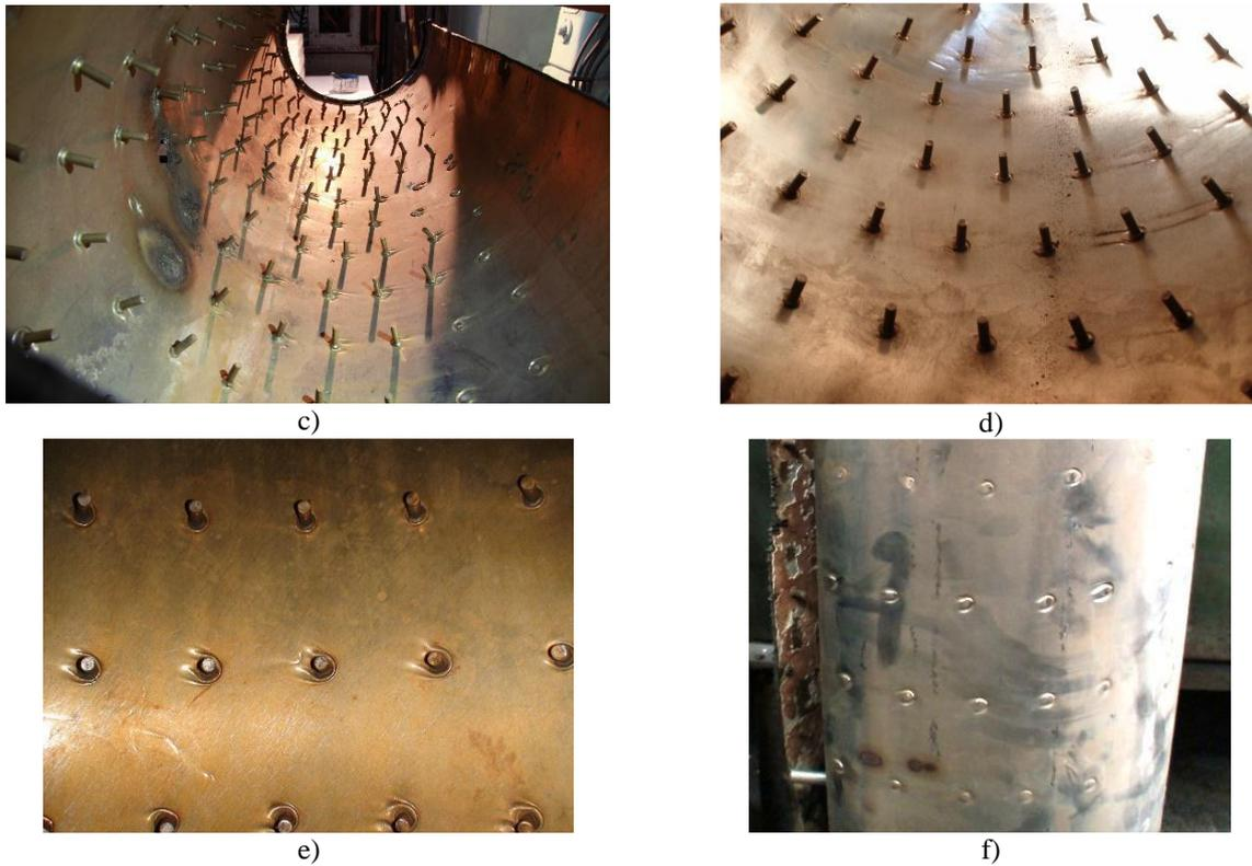
**Figure 2.3.** Spiral heat exchanger having defects along the entire width of the spirals, towards the center of the exchanger [30] a), b) overview of the spiral heat exchanger;
