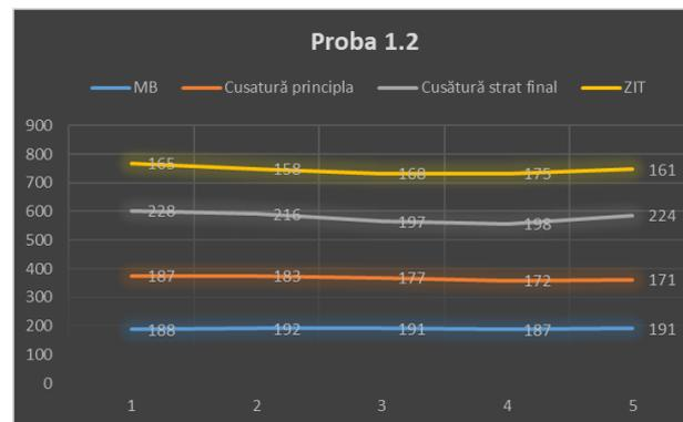
Figure 6.25. Hardness values graph for sample 1.2 [32]
