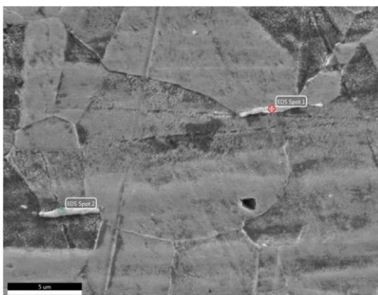
**Figure 6.19.** EDAX analysis on a microzone of the parent material (on delta ferrite islands)
