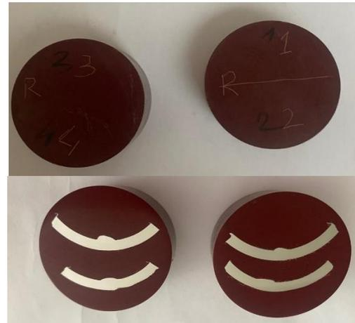
**Figure 6.9.** Sample 2 - positioning of welding points [33], 2.1. - point 1 - 50 mm; 2.2 - point 2 - 100m; 2.3. - point 3 - 150 mm; 2.4 - point 4 - 200 mm [33]
