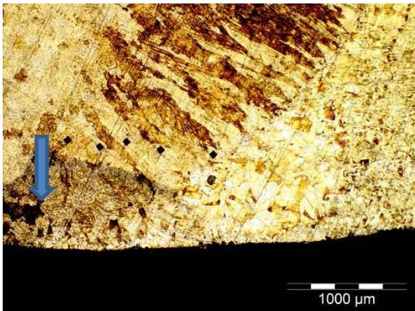
**Figure 6.16.** Welding root (50x)
