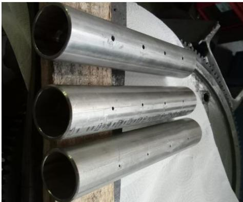
**Figure 5.1.** Austenitic stainless steel pipe X2CrNiMo17-12-2, 1÷3 samples [31, 33]
