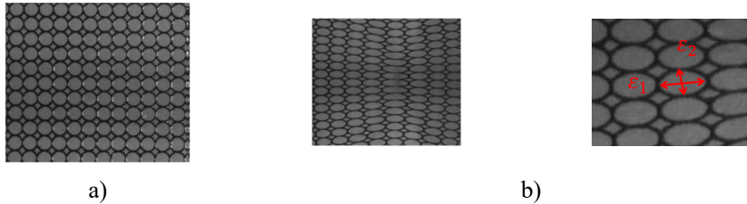
Fig. 1.1. Determination of major and minor principal strains values
