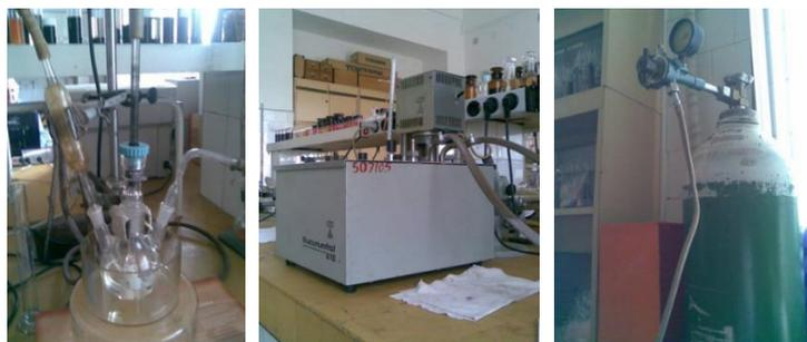
*Fig. 5.1: Installation in which the synthesis of magnetic nanoparticles took place: Mechanical stirrer; Thermostat and Nitrogen source under pressure*
