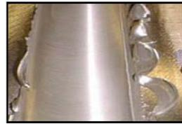
Fig. 2.3.2. Excessive burrs [B01]
