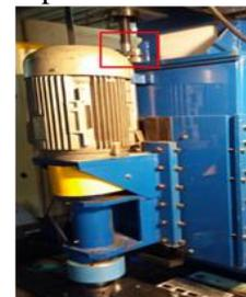
Fig. 6.2.7. Position of the force sensor in the experimental stand
