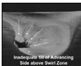
Fig. 2.3.5. Worm tunnel or hole [B01]
