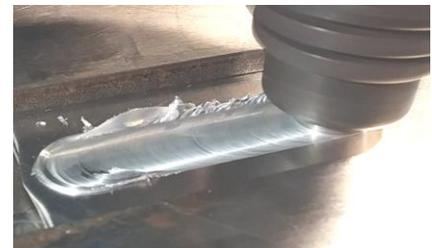
Fig. 9.2.11. The visual aspect of the welding seam made experimentally
