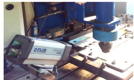
Fig. 6.2.4. Position of the thermographic chamber within the experimental stand
