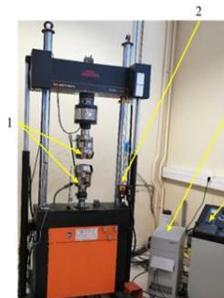
Fig. 6.11.1. INSTRON 1342 tensile test machine for traction/compression
