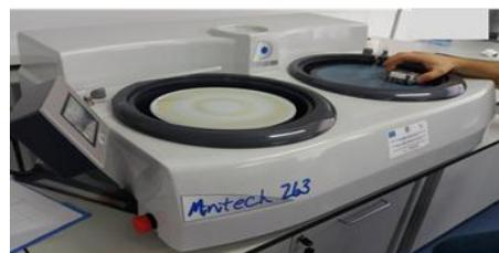
Fig. 6.7.2. Minitech 263 two-plate grinding machine
