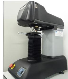
Fig. 6.10.1. INNOVATEST FALCON 500 microdurimeter
