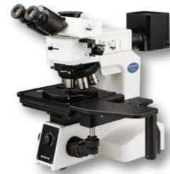
Fig. 6.9.2. OLYMPUS BX51M metallographic microscope
