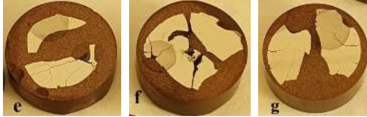
Figure VI.2.1 – High entropy alloys with biocompatible properties, included in epoxy resin, for optical microscopy (a- \text{FeTa}_{0.5}\text{Nb}_{0.5}\text{Ti}_{1.5}\text{Zr}_{0.5} ; b – \text{FeTa}_{0.5}\text{Nb}_{0.5}\text{TiZr}_{0.5} ; c – \text{FeMnNb}_{0.5}\text{TiZr}_{0.5} ; d - \text{FeTa}_{0.5}\text{Nb}_{0.5}\text{Ti}_{1.5}\text{Zr}_{0.5} remelted; e - \text{FeTa}_{0.5}\text{Nb}_{0.5}\text{Ti}_{1.5}\text{Zr}_{0.5} thermal treated; f – \text{FeTa}_{0.5}\text{Nb}_{0.5}\text{TiZr}_{0.5} thermal treated; g - \text{FeTa}_{0.5}\text{Nb}_{0.5}\text{Ti}_{1.5}\text{Zr}_{0.5} remelted and thermal treated)
