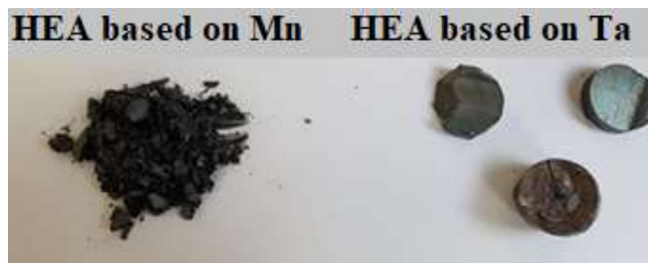
Figure V.3 – High entropy alloys with biocompatible properties samples after the application of homogenization annealing heat treatment
