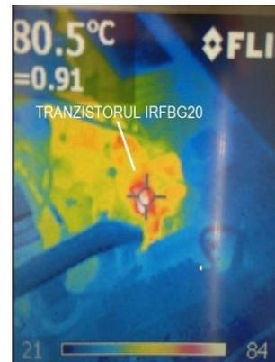
Figure 4.27. Temperature value of transistor with fan completely off [78]
