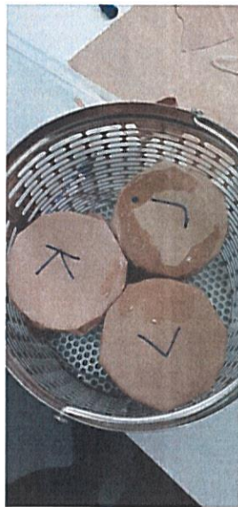
I. Autoclaving of MS/ZnO samples to fix the zinc oxide layer at a temperature of T = 110^{\circ} - 150^{\circ} \text{C} , t = 15 - 30 \text{ min}
