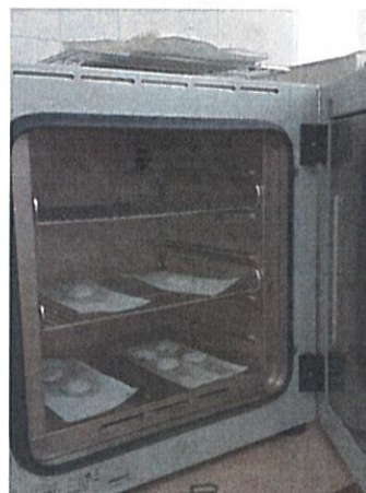
II. Oven drying of samples, Support Materials functionalized with ZnO (SpongeMat/ZnO), t = 24 \text{ h}
