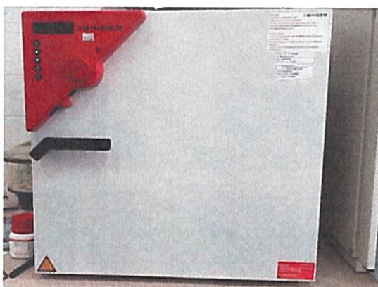
II. Oven drying of samples, Support Materials functionalized with ZnO (SpongeMat/ZnO), t = 24 \text{ h}
