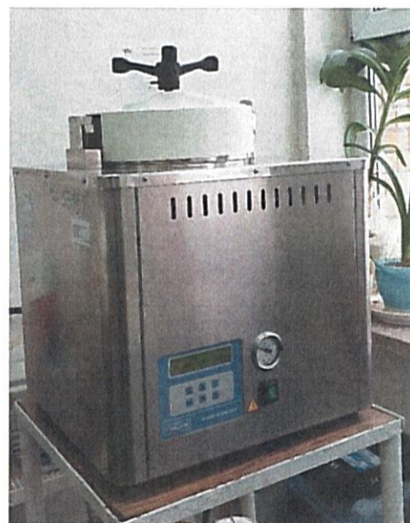
I. Autoclaving of MS/ZnO samples to fix the zinc oxide layer at a temperature of T = 110^{\circ} - 150^{\circ} \text{C} , t = 15 - 30 \text{ min}
