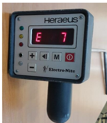
Fig.2.2. Portable immersion lance for temperature measurement
