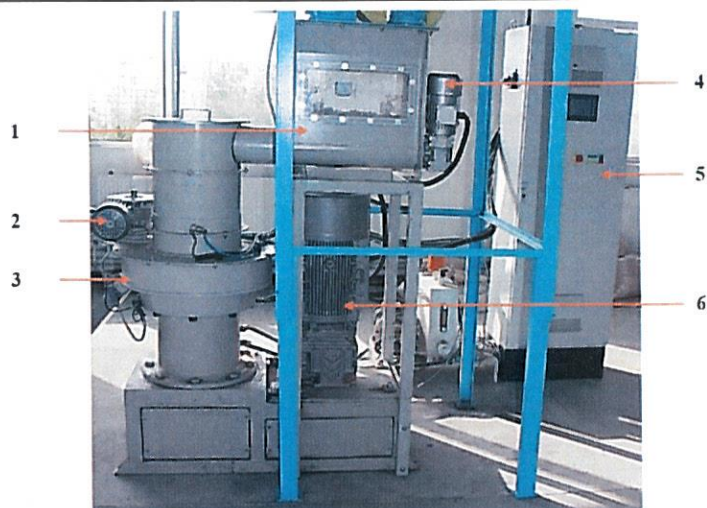
Fig. 6.6. Ring die pelleting equipment used to conduct the experiments 1. mini bunker for material feed; 2. Pellet curing blade motor; pelleting die casing; 4. feeding bunker motor; 5. Command panel; 6. Press main motor
