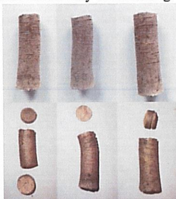
Fig. 5.19. Examples of pellets that disintegrated (broke) during evolution tracking sus – pellets on the day of obtaining; jos – disintegrated pellets
