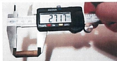
Fig. 5.17. Detail during pellet length measurements
