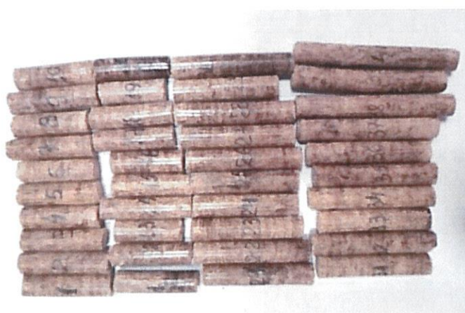
Fig. 6.7. Pellets obtained using the ring die pelleting machine
