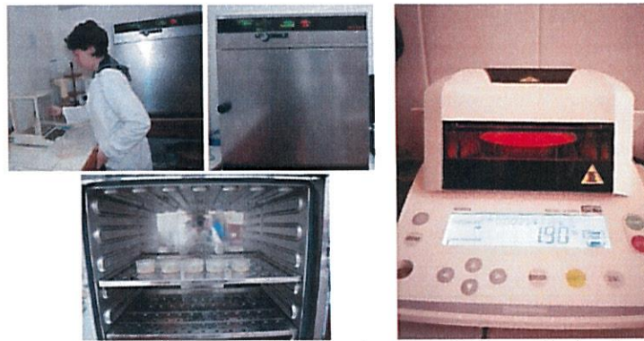
Fig. 5.2. Moisture determination for the samples in the oven (left) and in the thermobalance (right)
