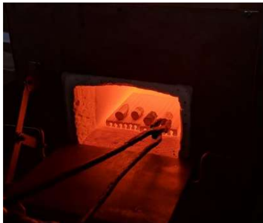
Fig. 4. 4 Heating the samples in the furnace to 1150°C
