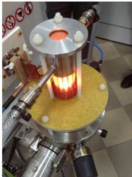
Fig. 4. 1 Induction furnace with cold crucible, vacuum and argon atmosphere
