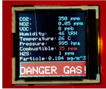
Figure. 6.5 Information shown on the display with an alarm that is triggered when a high concentration of flammable gas occurs
