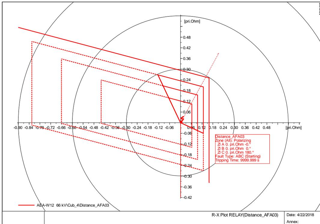
**Fig. 5. 3.** Characteristic of R-X plot of Distance\_AFA03 Relay
