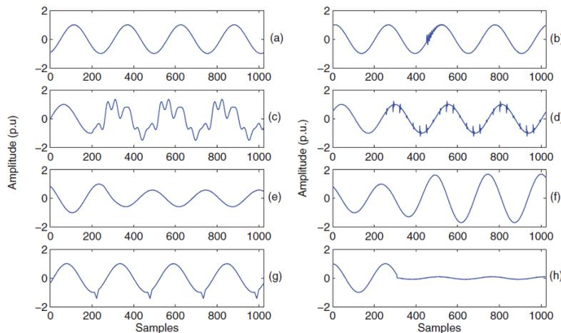
**Fig. 1. 1.** Examples of voltage signals and disturbances
