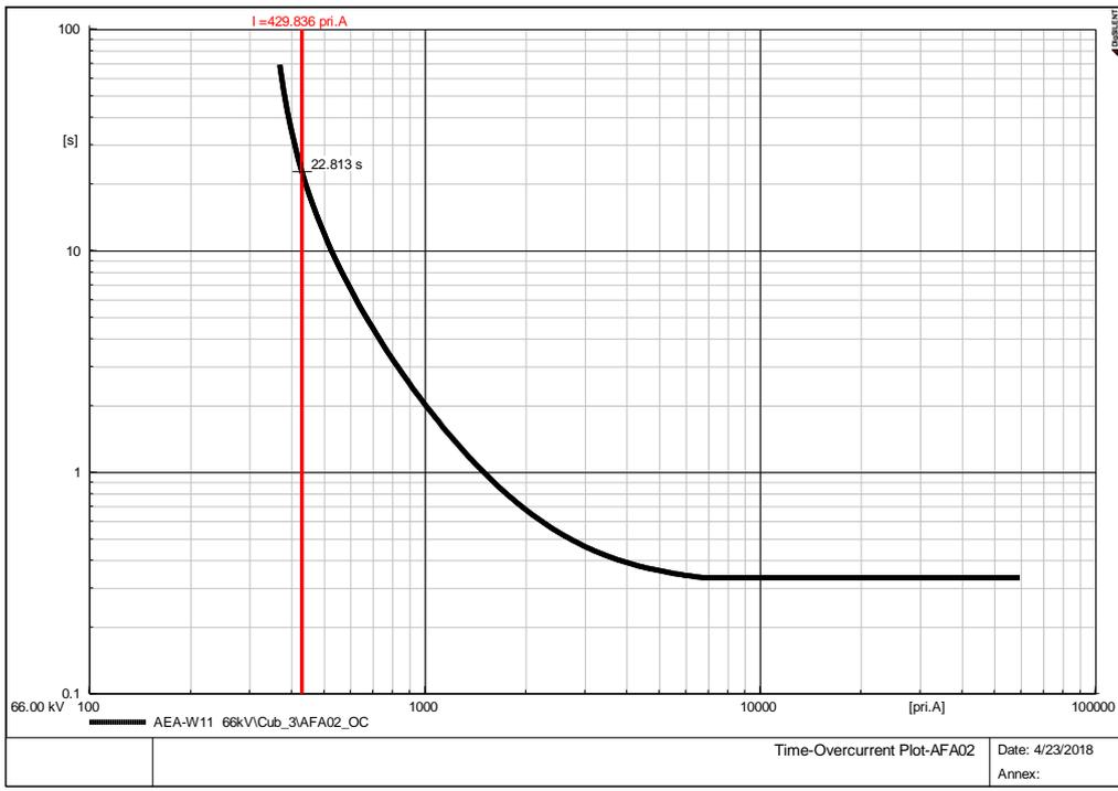
**Fig. 5. 6.** Time overcurrent plot \_ AFA02
