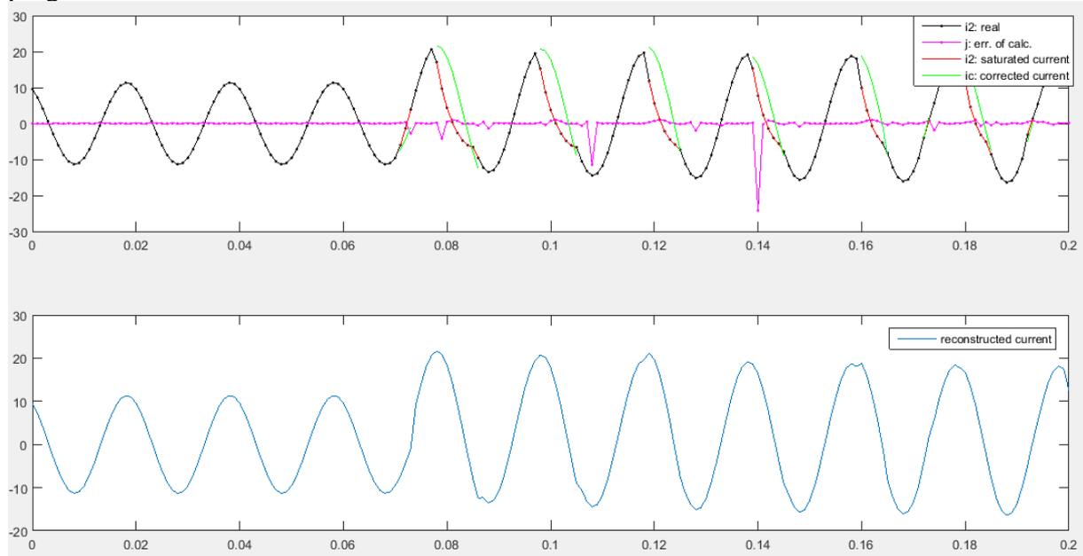
**Fig. 6. 7.** Corrected Current by using the proposed algorithm
