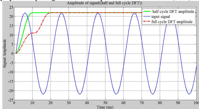
**Fig. 2. 2.** Input signal and its resultant amplitude by means of Fourier filter
