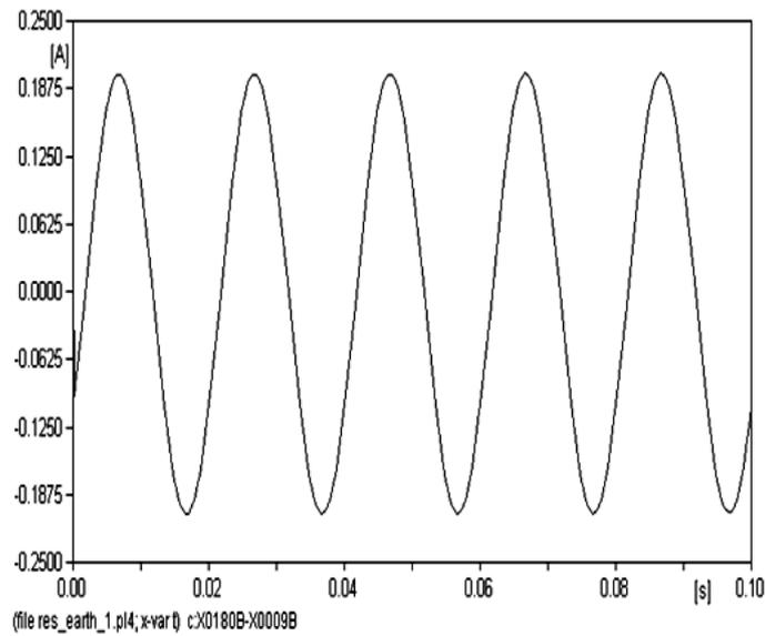
**Fig. 5. 18.** The differential current, passing in the phase (B)
