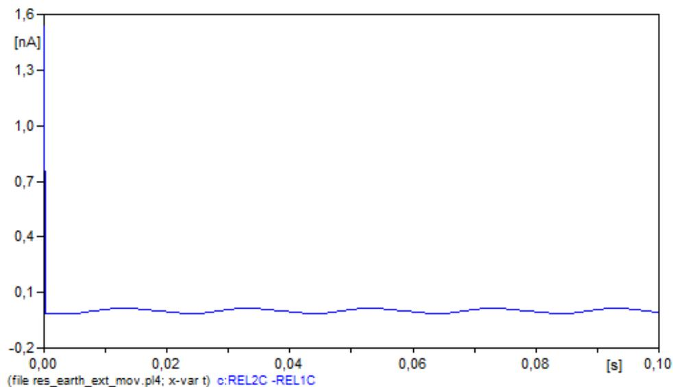
**Fig. 5. 23.** The differential current, passing in the phase (C)
