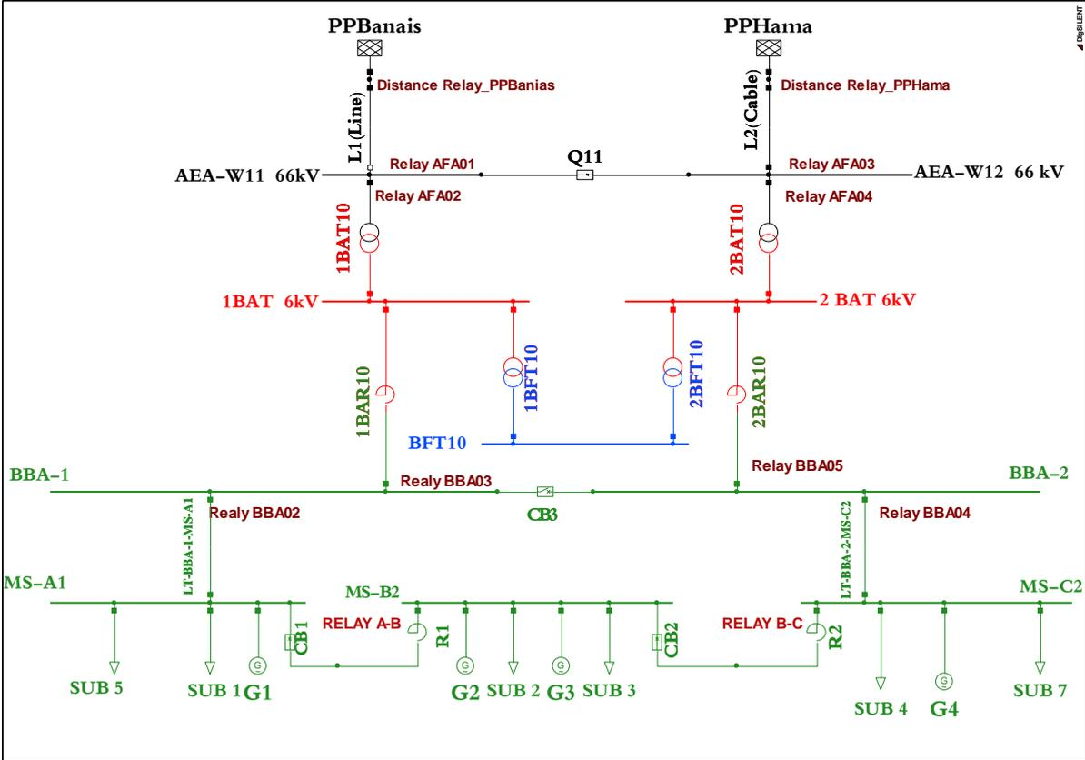
Fig. 4. 1. Distribution of relays for different elements of the studied power system
