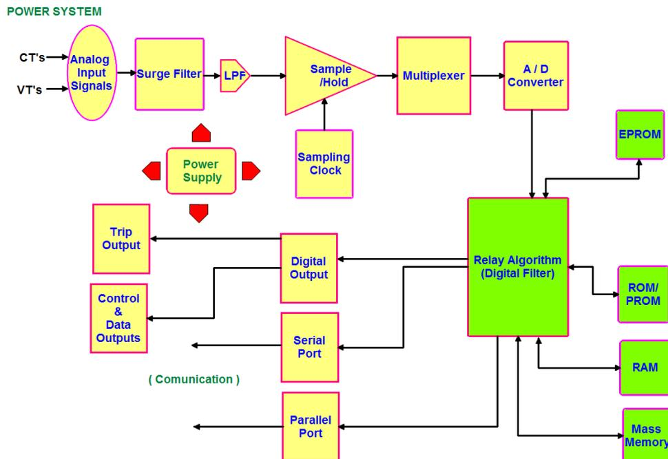
fig. 2. 1. Typical functional block diagram of a digital relay
