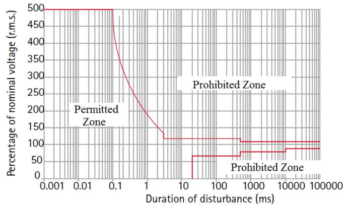
**Fig. 1. 3.** ITI curve for equipment Susceptibility
