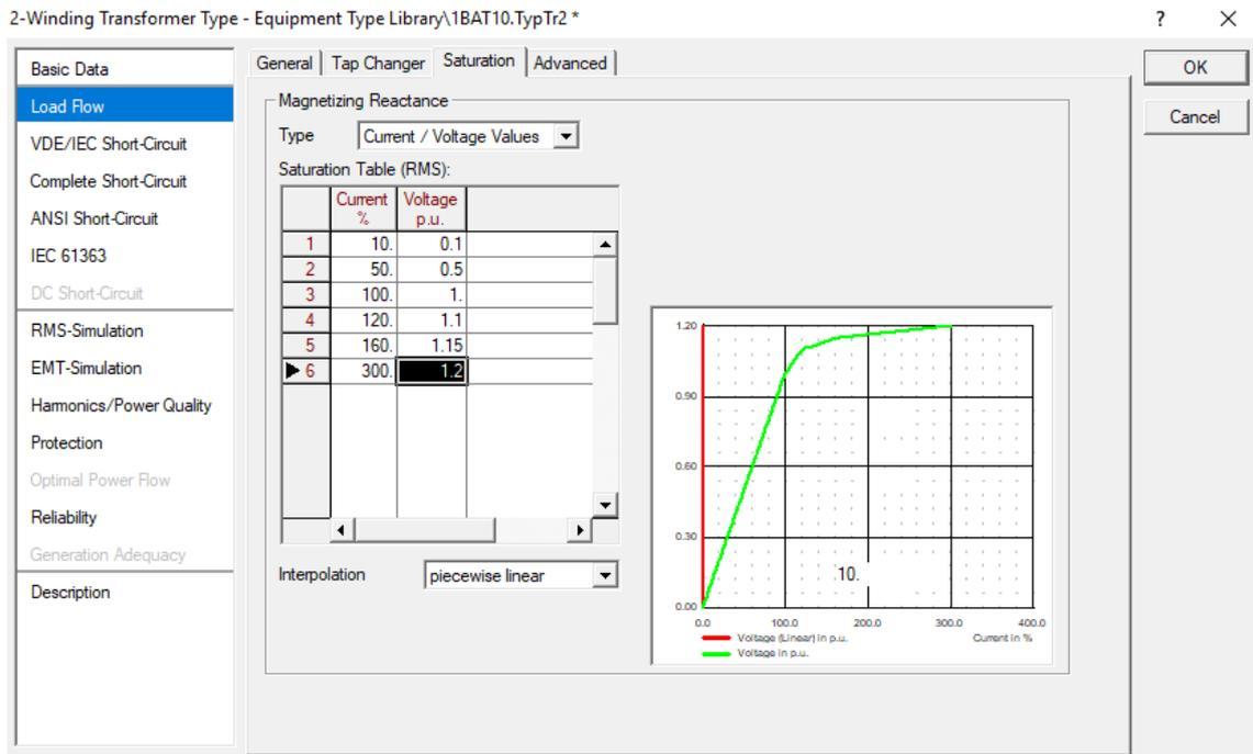
**Fig. 5. 4.** Magnetization curve of 1BAT 10
