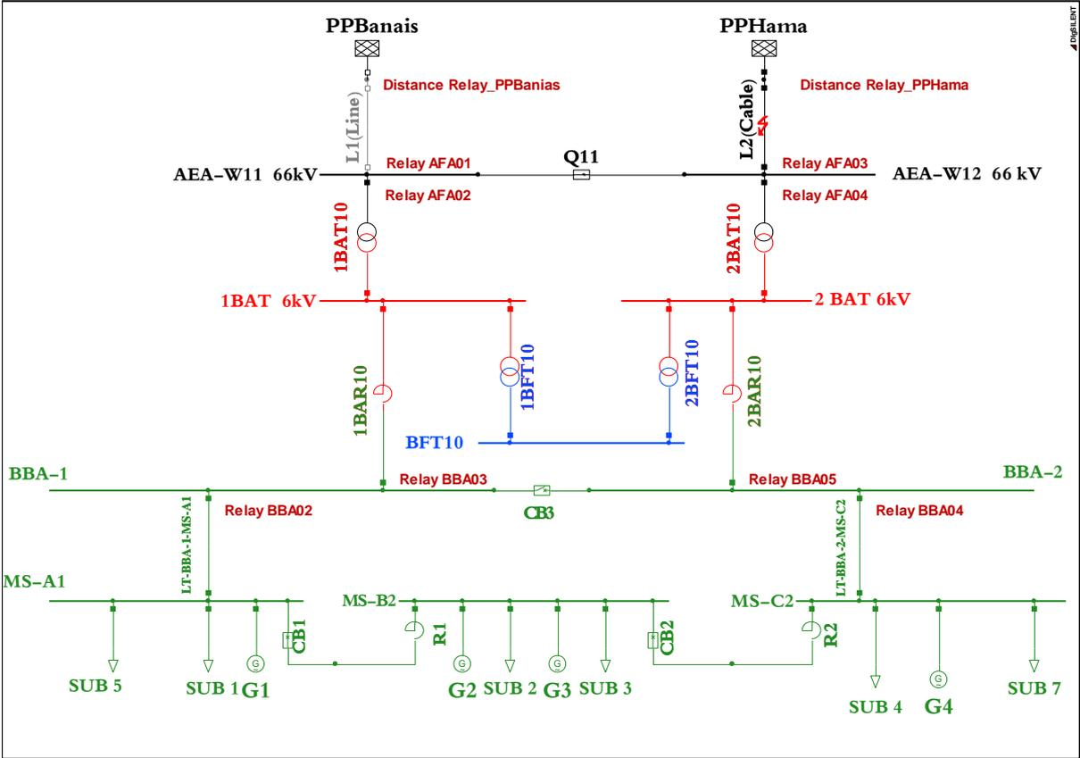
**Fig. 4. 2.** Three-phase fault at the distance 3.32 Km from Distance Relay\_PPHama
