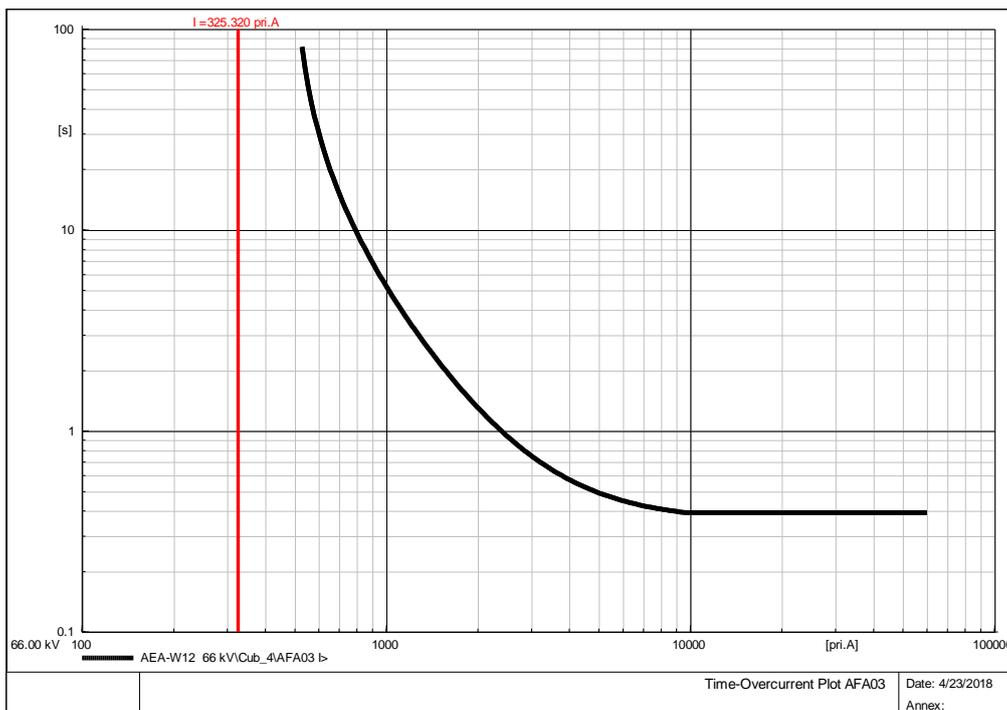
**Fig. 5. 10.** Time overcurrent plot \_ AFA03
