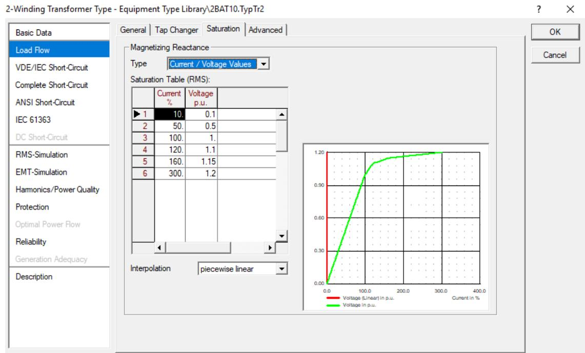
**Fig. 5. 5.** Magnetization curve of 2BAT 10
