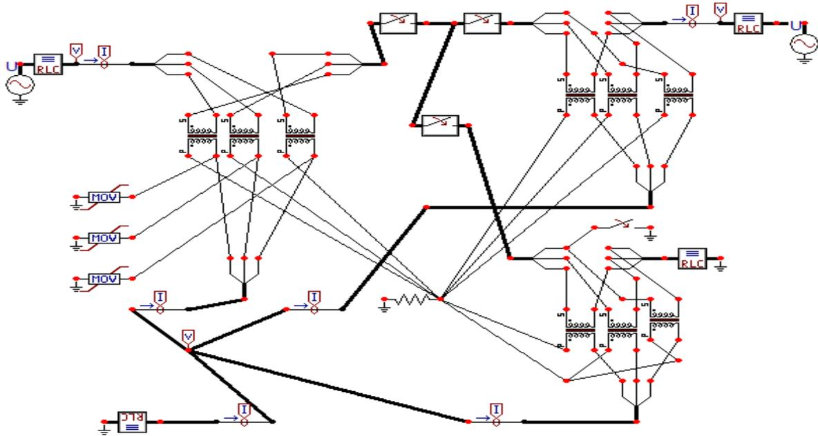
Fig. 5. 12. Representation of the power system in the case of internal fault by using EMTP-ATP
