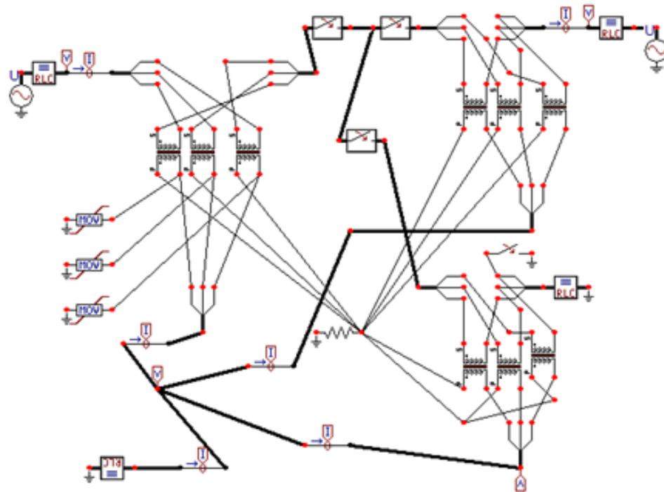
**Fig. 5. 20.** Representation of the power system in the case of an external fault
