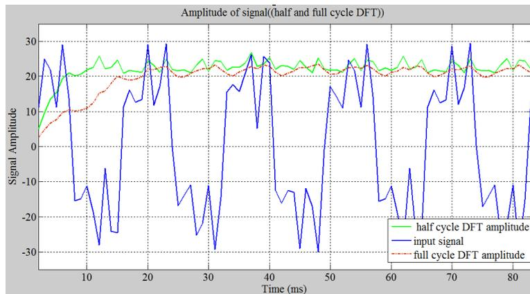
**Fig. 2. 7. Input signal and its resultant amplitude by means of Fourier filter**
