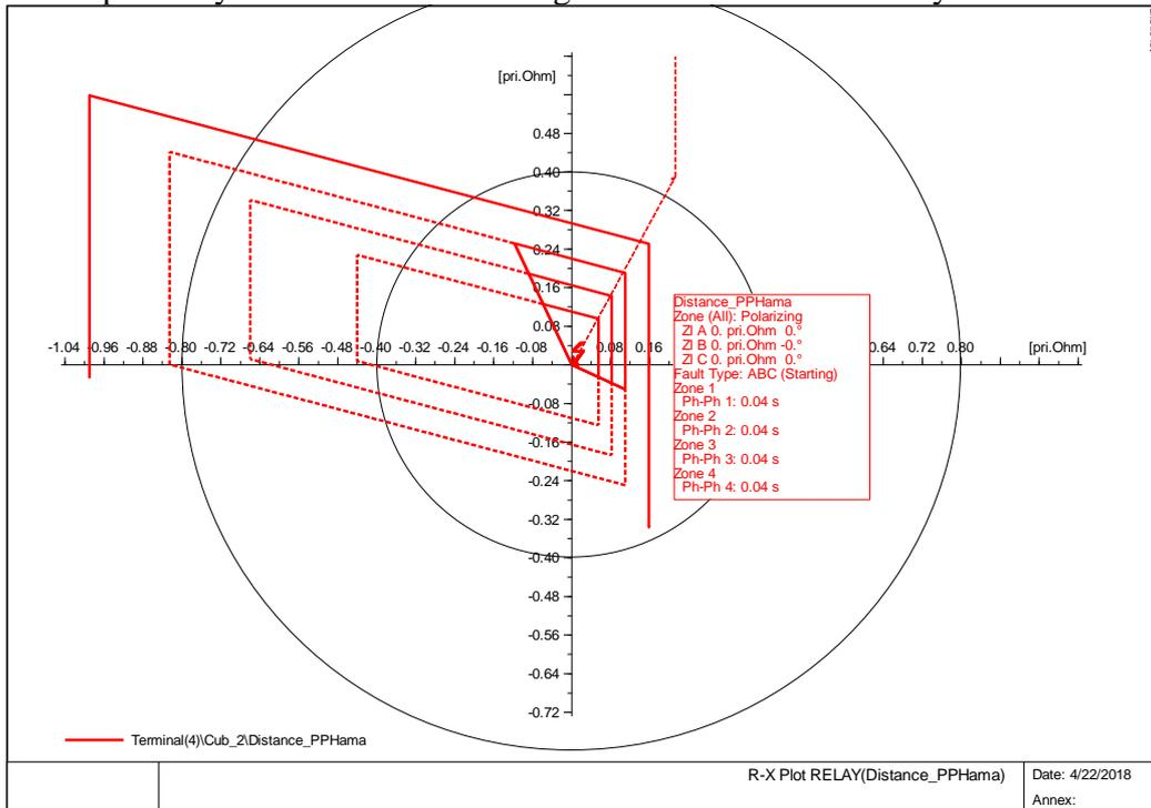
**Fig. 5. 2.** Characteristic of R-X plot of Distance\_PPHama
