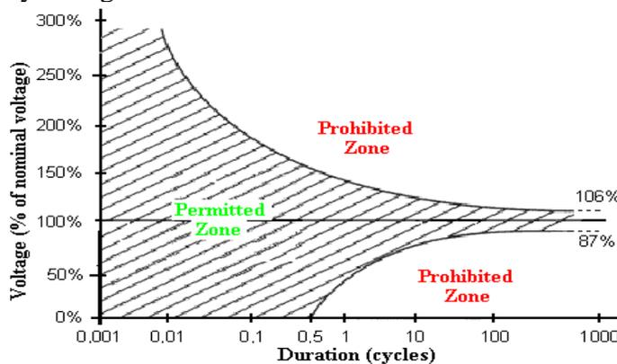
**Fig. 1. 2.** CBEMA curve for equipment Susceptibility
