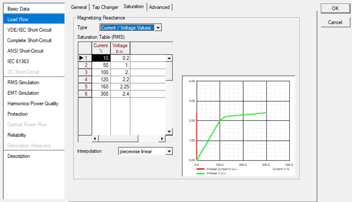
Fig. 5. 8. Magnetization curve of 1BAT 10
