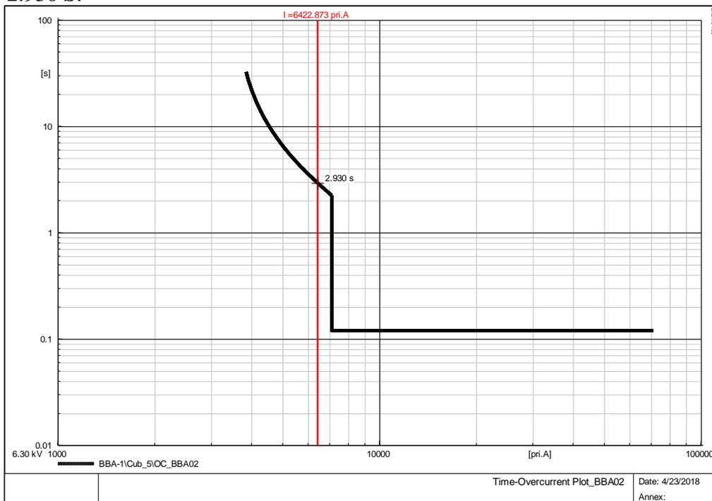
**Fig. 4. 8.** Time overcurrent Relay\_ BBA02 plot
