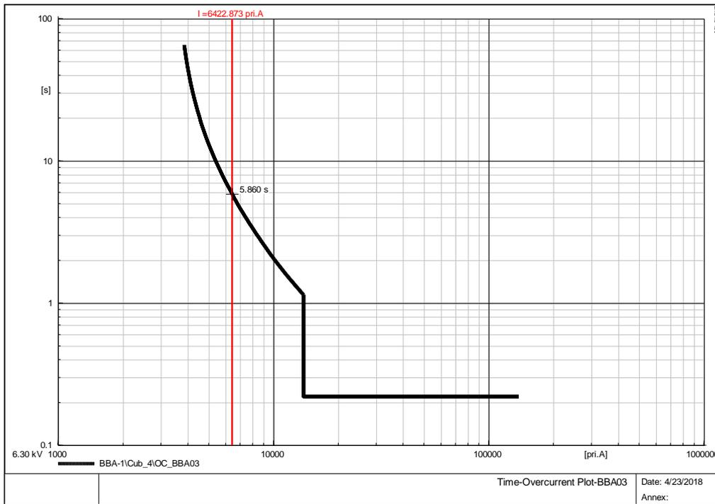
**Fig. 4. 7.** Time overcurrent Relay\_ BBA03 plot
