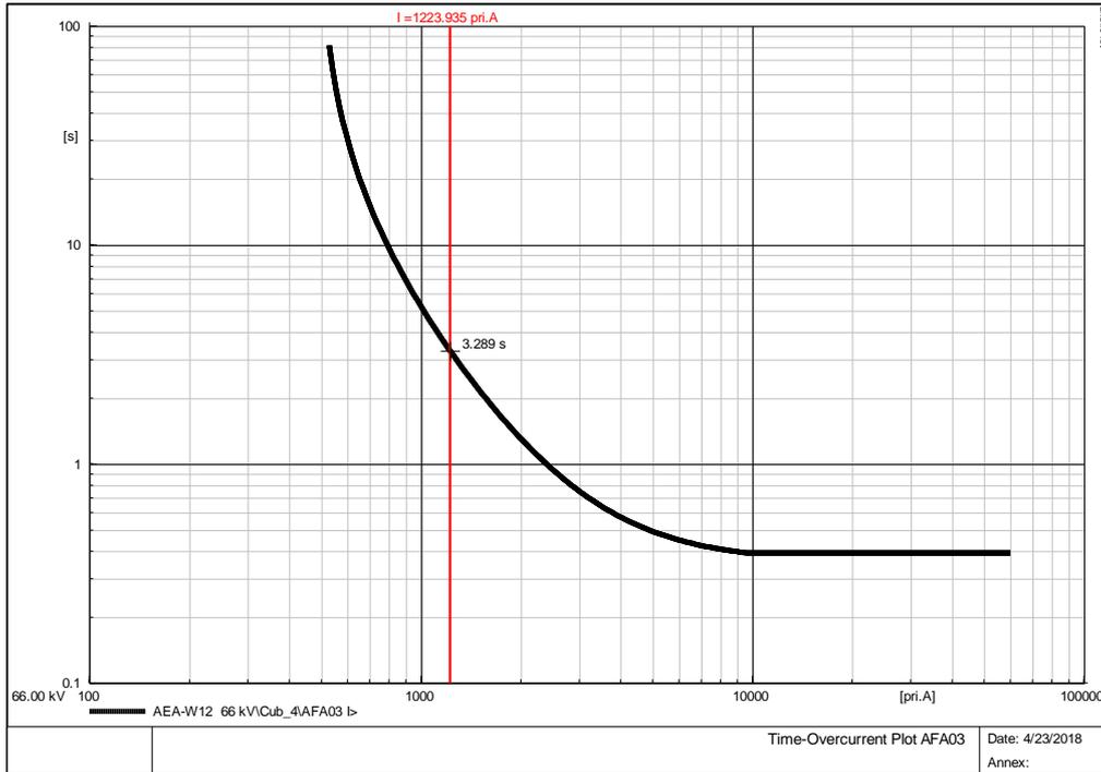
**Fig. 4. 5.** Time overcurrent Relay\_ AFA03 plot
