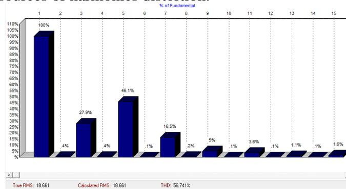
**Fig. 2. 6. Harmonics analysis of input signal by using Micom S1 Agile**
