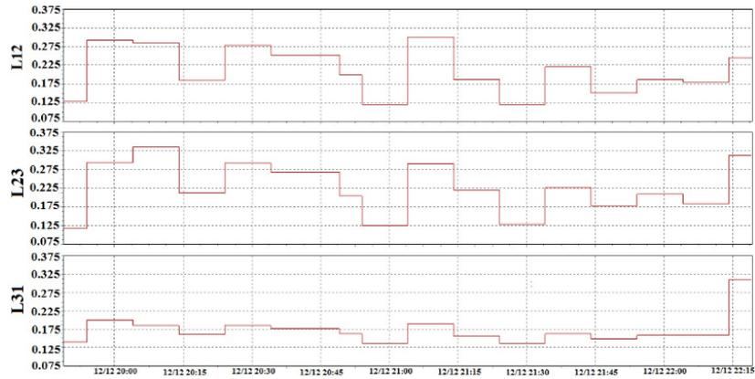
**Fig. 1. 5.** Voltage fluctuations (flickers)
