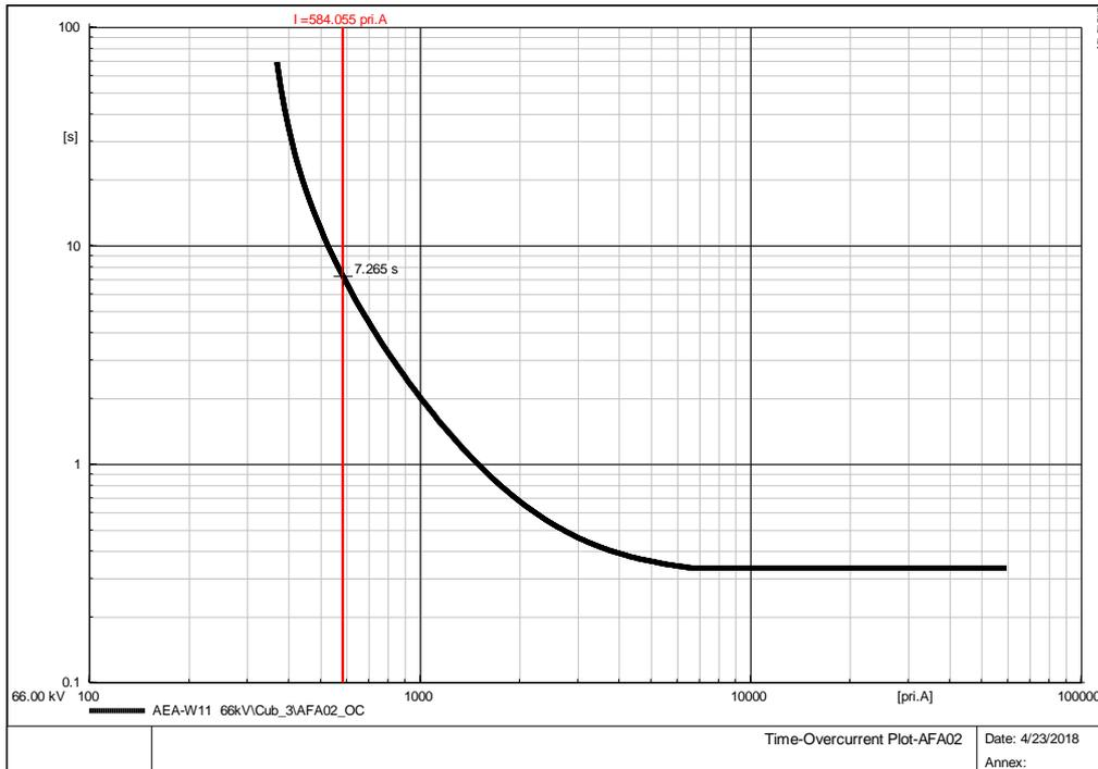
**Fig. 4. 6.** Time overcurrent Relay\_ AFA02 plot
