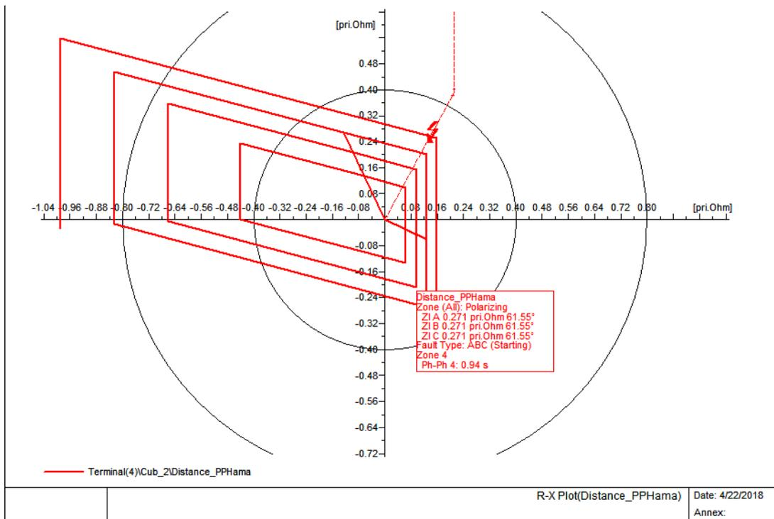
**Fig. 4. 3.** Characteristic of R-X plot of Distance\_PPHama Relay
