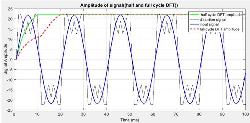
**Fig. 2. 3.** Input signal and its resultant amplitude by means of Fourier filters in case 2
