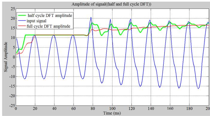
**Fig. 2. 5. Saturated wave current and its amplitude by using DFT**
