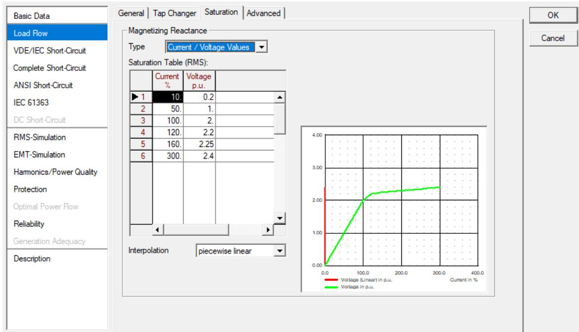
Fig. 5. 8. Magnetization curve of 2BAT 10
