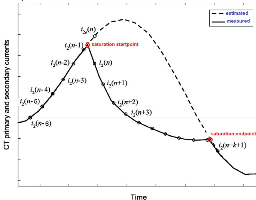
Fig. 6. 1. Real measured values and estimated values s of CT' secondary currents
