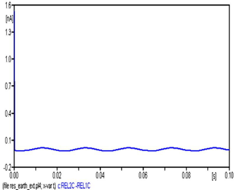
**Fig. 5. 15.** The differential current, passing in the phase (C)
