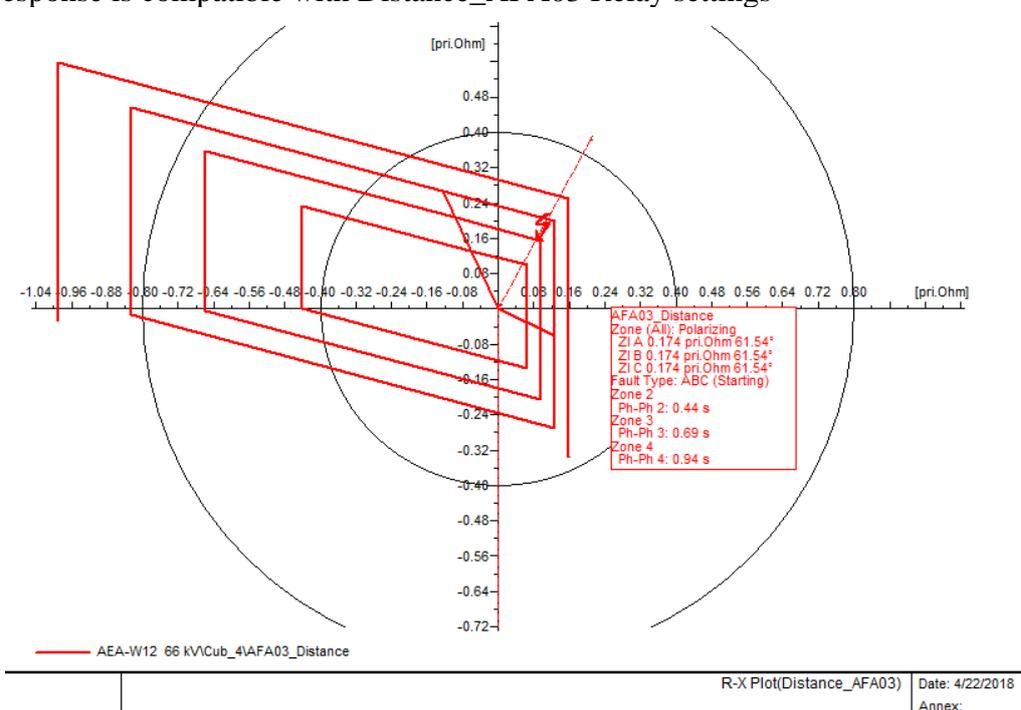
**Fig. 4. 4.** Characteristic of R-X plot of Distance\_AFA03 Relay
