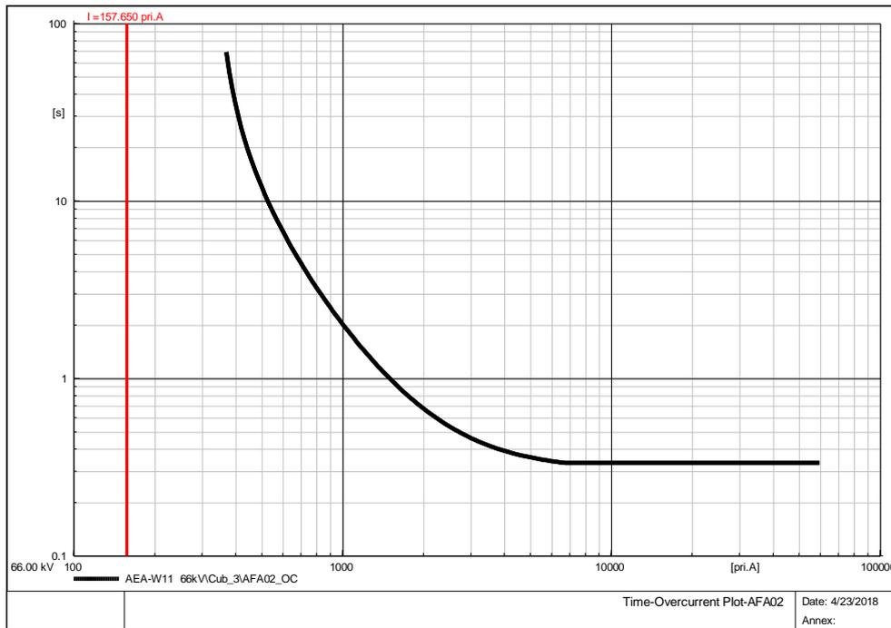
**Fig. 5. 9.** Time overcurrent plot \_ AFA02
