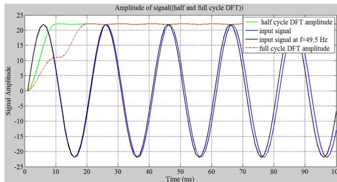
**Fig. 2. 4.** Input signal and its resultant amplitude by means of Fourier filters
