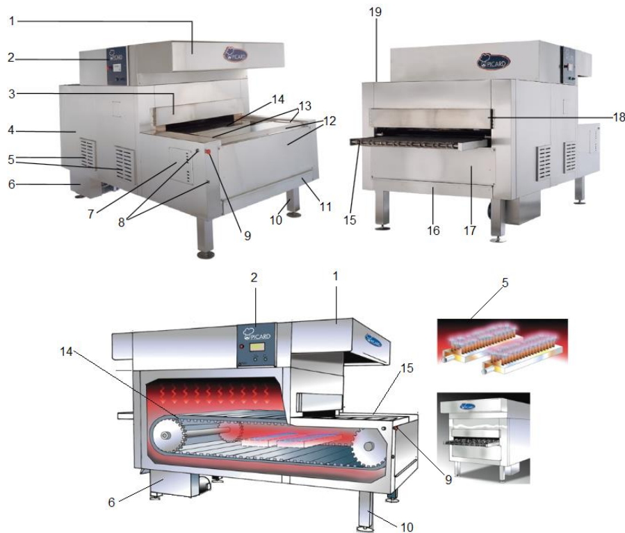
Fig. 3.5. Tunnel oven PICARD'S LP-200, [190]
