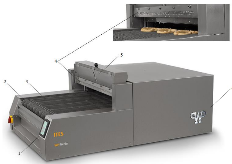
Fig. 3.6. Pretzel oven with infrared, [211]
