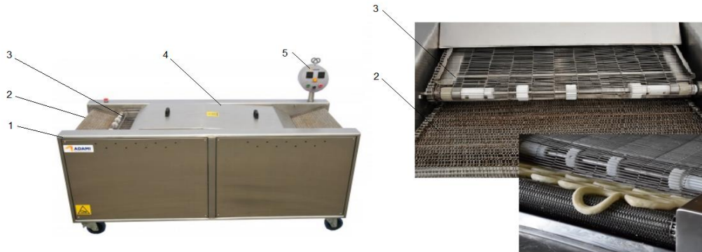
Fig. 3.4. Pretzel kettle - continuous, [11]
