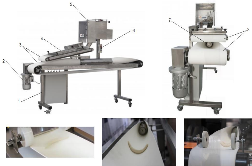
Fig.3.3. Pretzel shaper, model CO.FO 63/47, [192]
