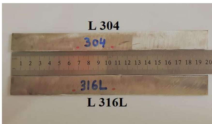
Fig. 5.1 Standard corrosion specimens of AISI 304 and AISI 316L austenitic stainless steels
