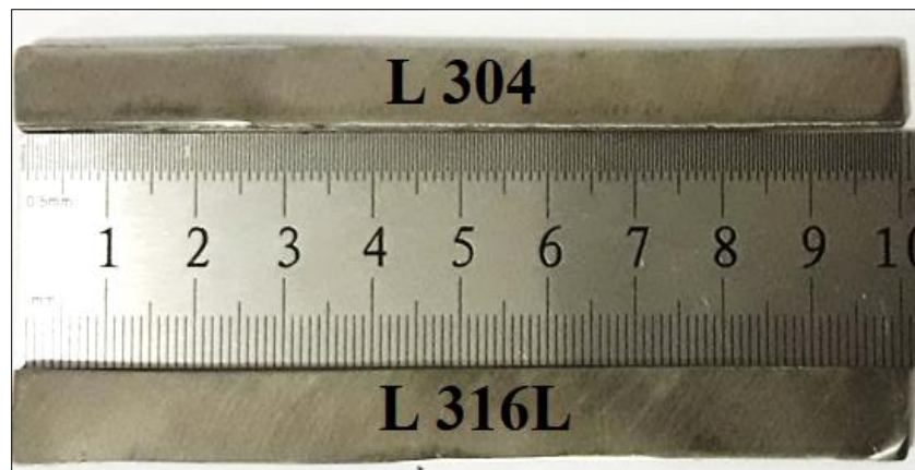
Fig. 6.2 Standard non-welded SCC specimens of AISI 304 and AISI 316L austenitic stainless steels
