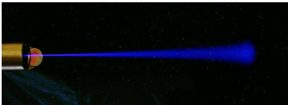
Figure 14: Long exposure picture of in-air proton beam
