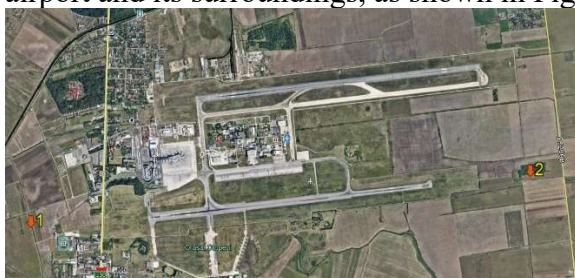
Figure 7.9 Points 1 and 2 where take-off noise measurements were made and aircraft landing respectively
