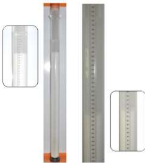
Fig. 5.2. Appearance of column with suspension during the experiment, [124]
