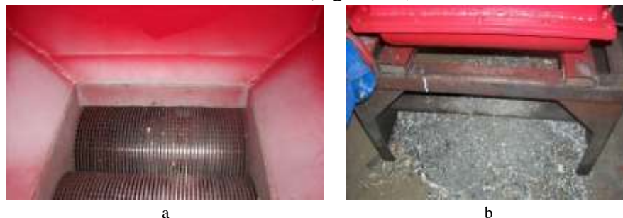
Fig. 6.56. Shreddings rotors fitted with cutting blades (a) and the appearance of the resulting shredding (b)
