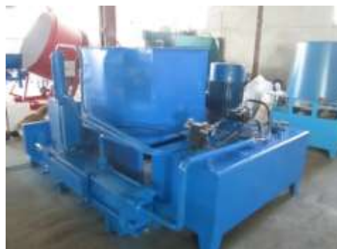
Fig. 6.59. Hydraulic press with piston for briquetting
