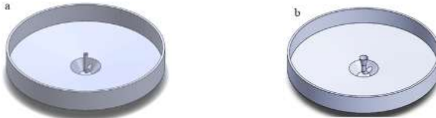
Fig. 5.10. Isometric view of a radial clarifier in a simplified structure in the case of a clarifier with a feeding pipe of constant diameter (a) or flared (b)
