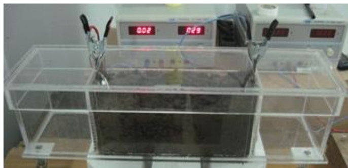
Fig. 4.2. Experimental installation used for electrochemical treatment application
