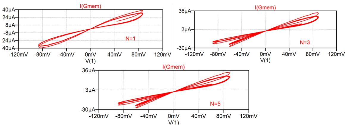
Figure 4.8 Hysteresis loop  $I_{Na}=f(V_{Na})$  for  $A=B=50mV$ ,  $N=1,3,5$ ,  $\Phi=\pi/3$
