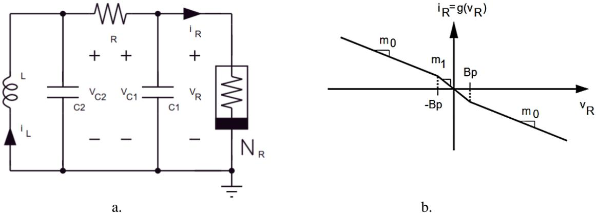
Figure 5.1 a Chua's chaotic oscillator. b.  $I$ - $V$  nonlinear characteristic of  $N_R$  circuit element [21]
