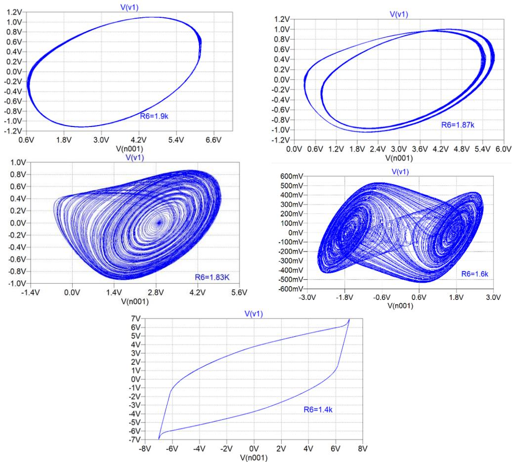
Figure 5.8 Typical bifurcation sequences encountered (horizontal axis  $V2$ , vertical axis  $V1$ ): (a)  $R6 = 1.9 k\Omega$  *period-1*, (b)  $R6 = 1.87 k\Omega$  *period-2*, (c)  $R6 = 1.83 k\Omega$  Chua's spiral attractor, (d)  $R6 = 1.6 k\Omega$  double-scroll attractor, (e)  $R6 = 1.4 k\Omega$  boundary crisis phenomenon.
