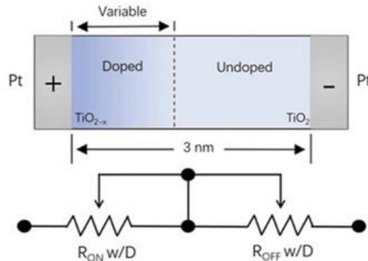
Figure 2.2 Internal structure of a memristor ( $w$  - variable width of the doped layer,  $D$  - total width of the memristor - 3nm for HP model) [3]
