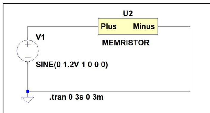
Figure 3.2 LTSpice analysis of a memristor
