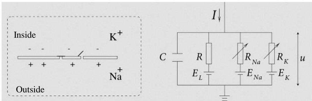
Figure 4.1 Electrical circuit of the Hodgkin Huxley model [19]
