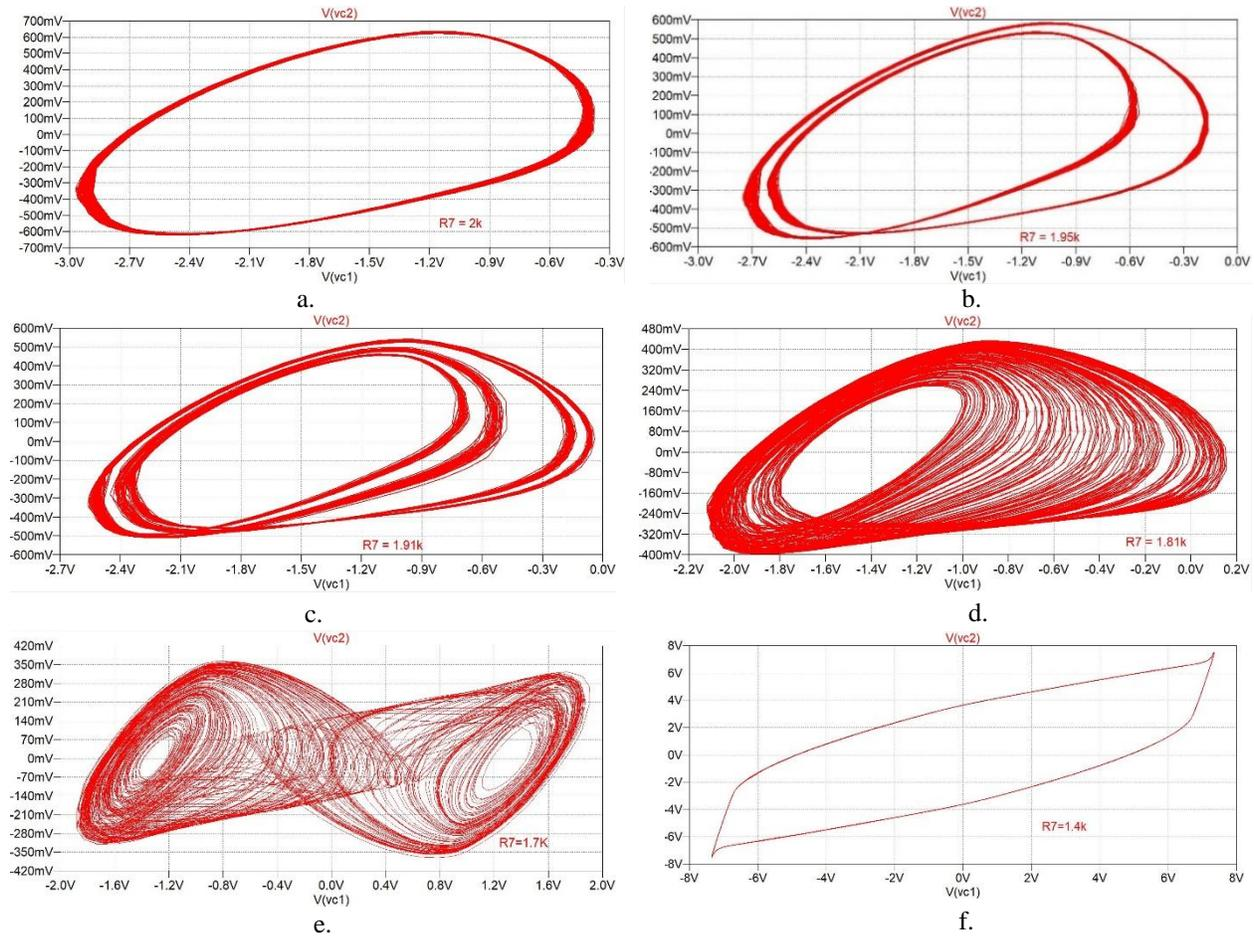
Figura 5.11. Typical bifurcation sequences encountered (horizontal axis  $V_2$ , vertical axis  $V_1$ ): (a)  $R_7 = 2\text{ k}\Omega$  period-1, (b)  $R_7 = 1.95\text{ k}\Omega$  period -2, (c)  $R_7 = 1.83\text{ k}\Omega$  period -4, (d)  $R_7 = 1.72\text{ k}\Omega$  Chua's spiral attractor, (e)  $R_7 = 1.6\text{ k}\Omega$  double scroll attractor, (f)  $R_7 = 1.4\text{ k}\Omega$  boundary crisis phenomenon.
