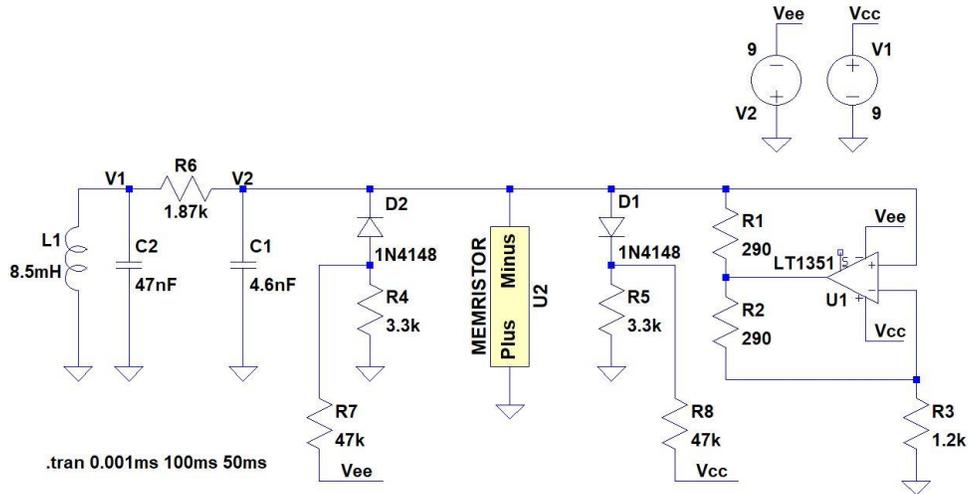
Figure 5.4 LTSpice topology of memristive oscillator
