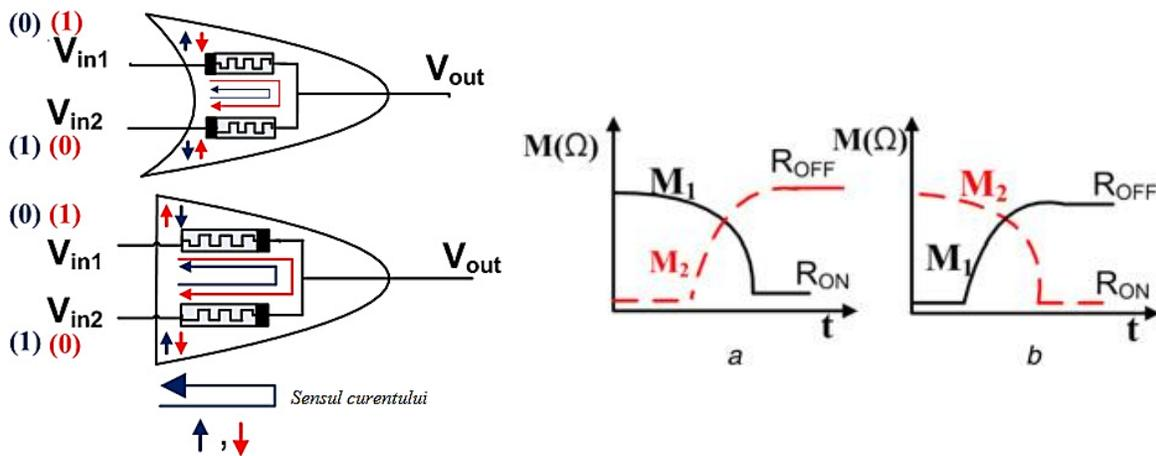
Figure 3.5 Logic gates with memristors. Memristance variation for OR (a), AND (b) logic gates [7]
