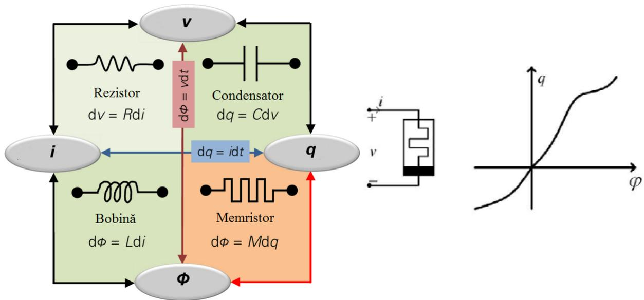
Figure 2.1 Passive circuit elements with two terminals [3]
