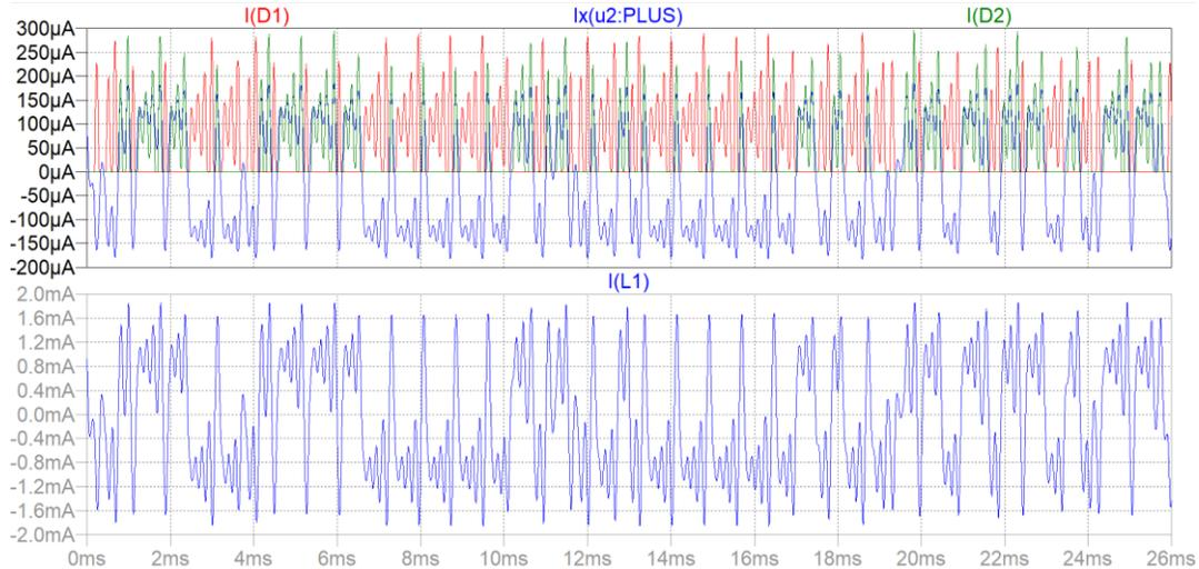
Figure 5.9 a) Electrical current for  $D1$ ,  $D2$ , Memristor components
