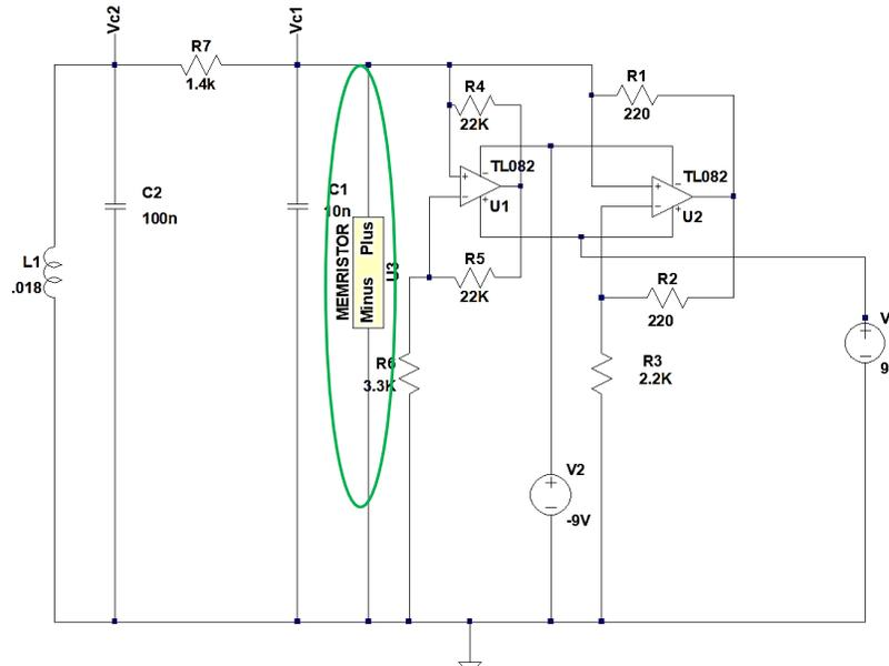
Figure 5.10 Chua's memristive oscillator circuit topology, implemented in LTSpice
