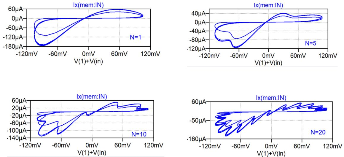
Figure 4.6 Hysteresis loop  $I_k=f(V_k)$  for  $A=50\text{mV}$ ,  $B=10\text{mV}$ ,  $N=1,5,10,20$
