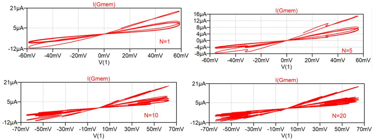
Figure 4.9 Hysteresis loop  $I_{Na}=f(V_{Na})$  for  $A=50\text{mV}$ ,  $B=15\text{mV}$ ,  $N=1,5,10,20$ ,  $\Phi=\pi/3$
