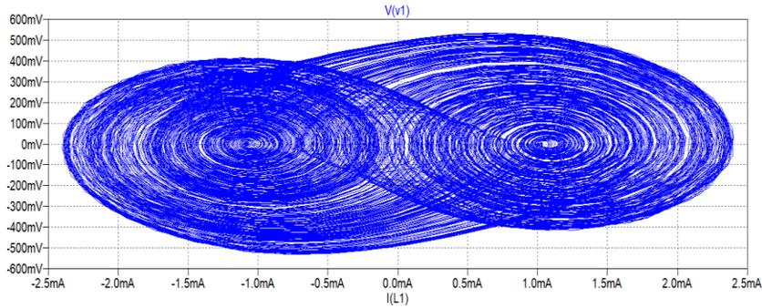
Figure 5.7 Double scroll attractor  $I=f(V)$  for the memristive oscillator
