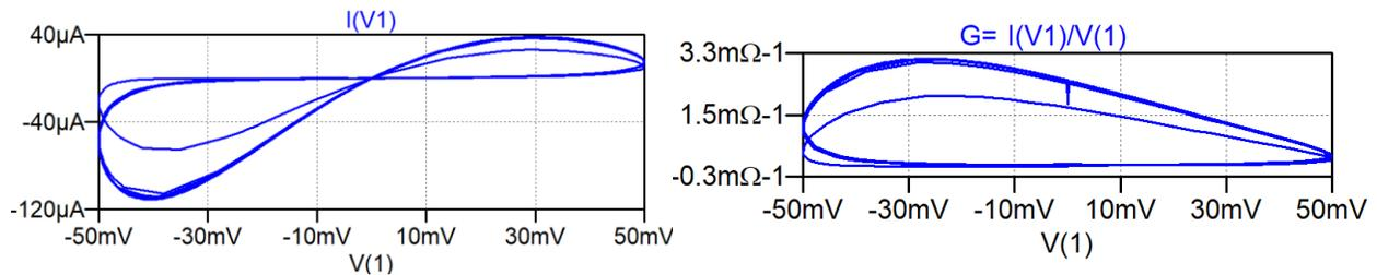
Figure 4.4 Hysteresis loop  $I_k=f(V_k)$ . Memconductance variance  $G_K$  vs. the supply voltage  $v_K$ .
