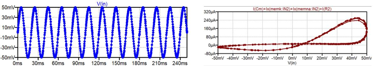
Figure 4.18 Supply voltage waveform and hysteresis loop of the memristive system  $I_m = f(V_{in})$
