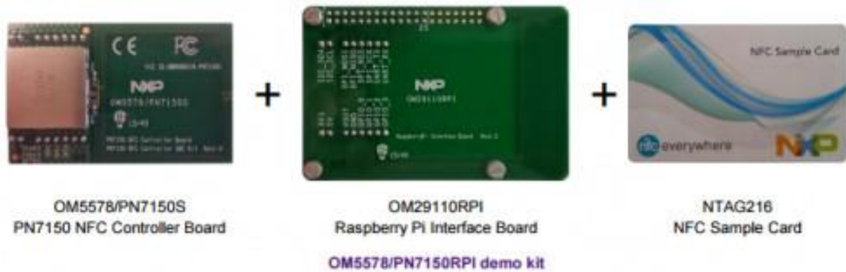
Fig VI-3 Cititor / Programator de carduri NFC OM5578 / PN7150 [31]
