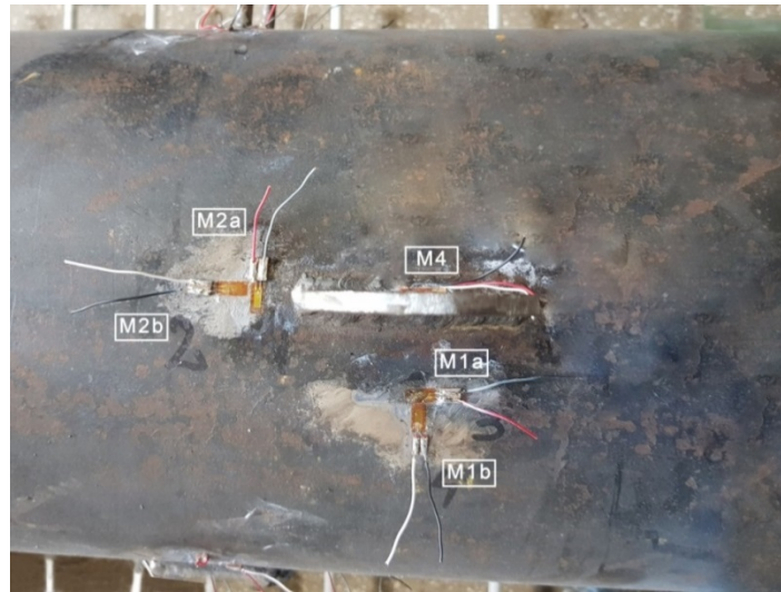
Fig. 6. 9. Positioning strain gauges around a flat lug
