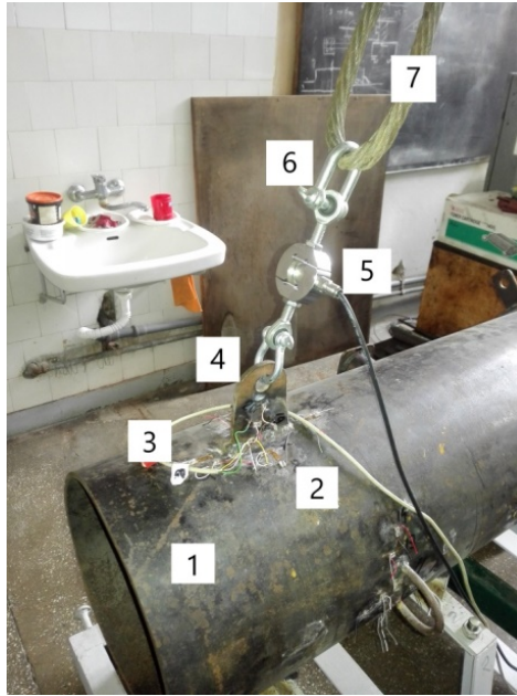
Fig. 6. 6. View from the grip area of an ear on the cylindrical body 1 – cylinder; 2 – strain gauges; 3 – electric circuit; 4 – lug for anchoring; 5 – force transducer; 6 – schackle; 7 - cable
