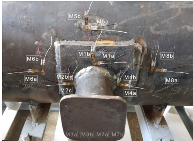
Fig. 6. 32. The experimental device with cylindrical trunnions
