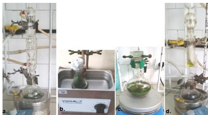
Figure 5.1. Installations for obtaining extracts from ivy leaves : a) refluxation, b) ultrasonication, c) maceration and d) Soxhlet extraction.
