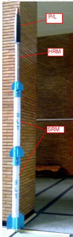
Fig. 1. Lansator suborbital de testare – SLT expus POLIFEST 2015
