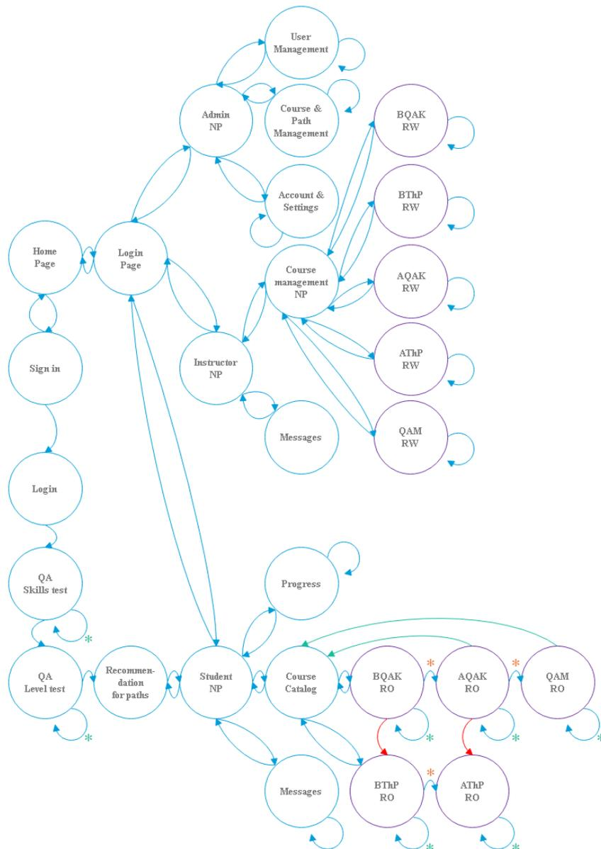
**Fig. 3.1** The transition state diagram of the e-learning application
