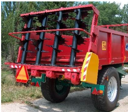
Fig. 3.24. Fertilizer spreader with 4 vertical beaters with continuous coil [90]
