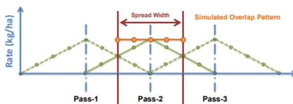
Fig.4.14. Graphical representation of overlapping three passes' patterns [105]
