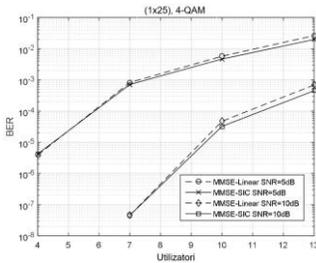
**Fig. 5.6** Linear MMSE and MMSE-SIC, RSZ equal to 5 dB and 10 dB, 4-QAM, base station with 25 antennas depending on the number of users
