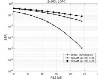
**Fig. 5.14** BER versus RSZ with LDPC for 50 active users, in a MIMO configuration of  $(2 \times 100)$
