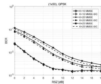
**Fig. 6.18** BER versus RSZ in a Massive (1x50) MIMO configuration, with LDPC and QPSK modulation, when the number of active users is equal to 10, 20, 25
