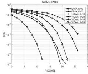
**Fig. 5.2** BER versus RSZ for a MIMO configuration of (2x50)
