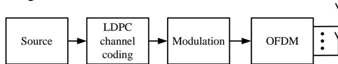
**Fig. 5.1** The data transmission
