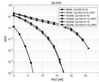
**Fig. 5.12** BER versus RSZ with and without LDPC for 10 active users, in a MIMO configuration of  $(2 \times 100)$
