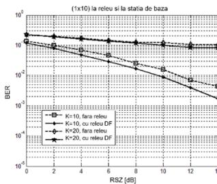
**Fig. 6.6** System performance when there are 10 antennas at the base station and 10 antennas at the relay, DF protocol
