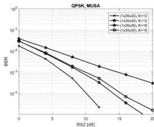
**Fig. 7.4** BER versus RSZ for (1x26x30) and (1x30x30) MIMO Massive configurations, QPSK modulation, MUSA with 12,16 active users
