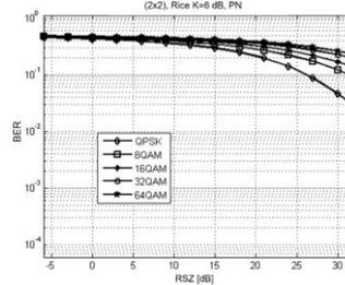
**Fig. 4.16** BER versus RSZ, QPSK and M-QAM ( $M = 8,16,32,64$ ), (2x2) MIMO, fading Rice,  $K = 6$  dB
