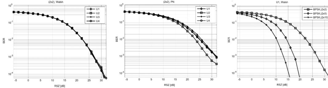
**Fig. 4.5** BER versus RSZ for BPSK, (2x2) MIMO, Walsh spreading codes
