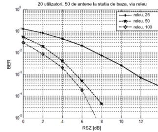
**Fig. 6.10** System performance when at the base station are 50 antennas and 20 active users, DF protocol
