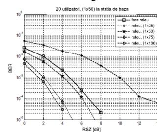
**Fig. 6.7** System performance when at the base station are 50 antennas and 20 active users, DF protocol
