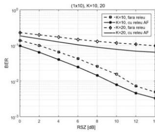
**Fig. 6.2** Massive MIMO system with multiple users in configuration (1x10) with and without relay, AF protocol
