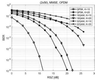
**Fig. 5.4** BER versus RSZ in a MIMO configuration of (2x50), in the presence of OFDM
