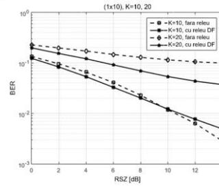
**Fig. 6.3** Massive MIMO system with multiple users in configuration (1x10) with and without relay, DF protocol
