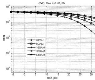
**Fig. 4.15** BER versus RSZ, QPSK and M-QAM ( $M = 8,16,32,64$ ), (2x2) MIMO, fading Rice,  $K = 3$  dB
