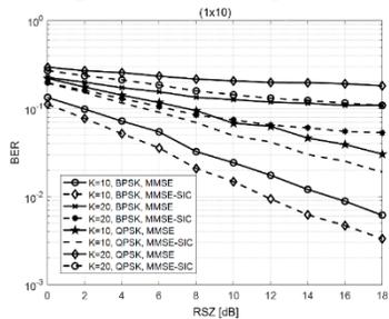
**Fig. 6.14** BER versus RSZ, (1x10) MIMO Massive, with LDPC, when the number of active users is equal to 10 and 20
