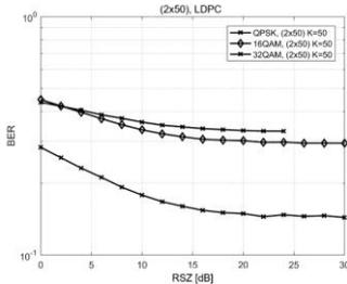
**Fig. 5.13** BER versus RSZ with LDPC for 50 active users, in a MIMO configuration of  $(2 \times 50)$
