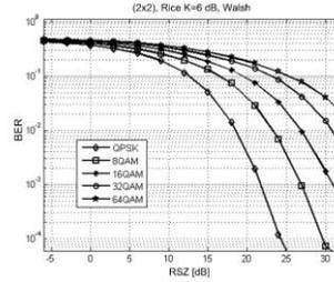
**Fig. 4.10** BER versus RSZ for QPSK and M-QAM ( $M = 8,16,32,64$ ), (2x2) MIMO, Fading Rice,  $K = 6$  dB
