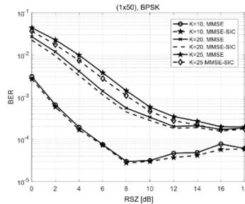
**Fig. 6.17** BER versus RSZ in a Massive MIMO (1x50) configuration, with LDPC and BPSK modulation, when the number of active users is equal to 10, 20, 25
