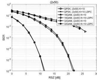
**Fig. 5.11** BER versus RSZ with and without LDPC for 10 active users, in a MIMO configuration of  $(2 \times 50)$
