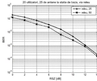
**Fig. 6.9** System performance when at the base station are 25 antennas and 20 active users, DF protocol
