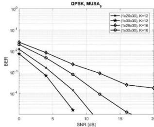
**Fig. 7.5** BER versus SNR for (1x26x30) and (1x30x30) MIMO Massive configurations, QPSK modulation, MUSA<sub>0</sub> with 12,16 active users
