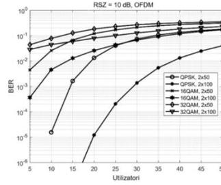
**Fig. 5.5** BER versus the number of users for RSZ = 10 dB, in the presence of OFDM
