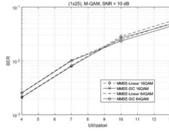
**Fig. 5.7** Linear MMSE and MMSE-SIC, RSZ equal to 10 dB, 16-QAM and 64-QAM, base station with 25 antennas depending on the number of users
