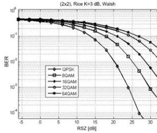
**Fig. 4.9** BER versus RSZ for QPSK and M-QAM ( $M = 8,16,32,64$ ), (2x2) MIMO, fading Rice,  $K = 3$  dB
