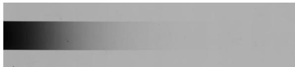
Figure 2.7: An example of RCF scan image. The irradiated region is placed in the middle side, between two non-irradiated regions. The RCF OD variation (from left to right) is based on the scattering cross-section of a proton beam on a Tantalum foil. The cross-section of the beam inside the target was estimated with the Rutherford formalism for elastic scattering.
