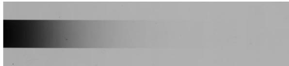
Figure 2.7: An example of RCF scan image. The irradiated region is placed in the middle side, between two non-irradiated regions. The RCF OD variation (from left to right) is based on the scattering cross-section of a proton beam on a Tantalum foil. The cross-section of the beam inside the target was estimated with the Rutherford formalism for elastic scattering.
