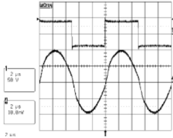
(b) Experimental results with Voltage (Top) 50V/div and current (Bottom) with 5A/div [2]
