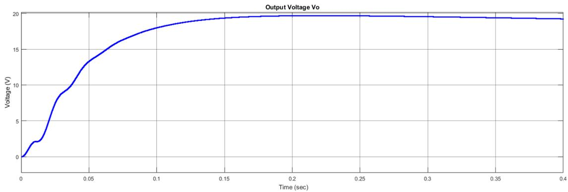
Figure 42- Output Voltage in mode 1
