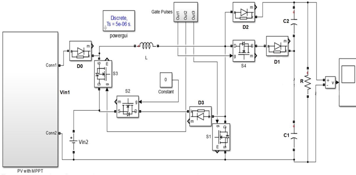
Figure 6-Dual Input Single Output Converter
