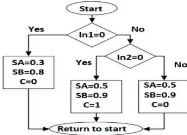
Figure 32- Flow chart for the controller operation
