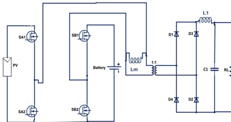
*Figure 19-Modified Full Bridge Three port converter*
