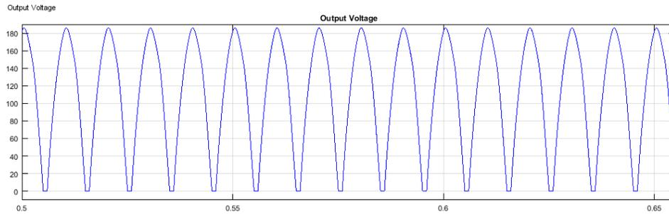
Figure 9-Output voltage of modified FB-TPC
