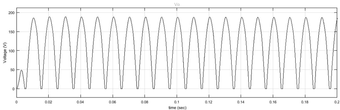
Figure 5-Output Voltage of three port full bridge converter
