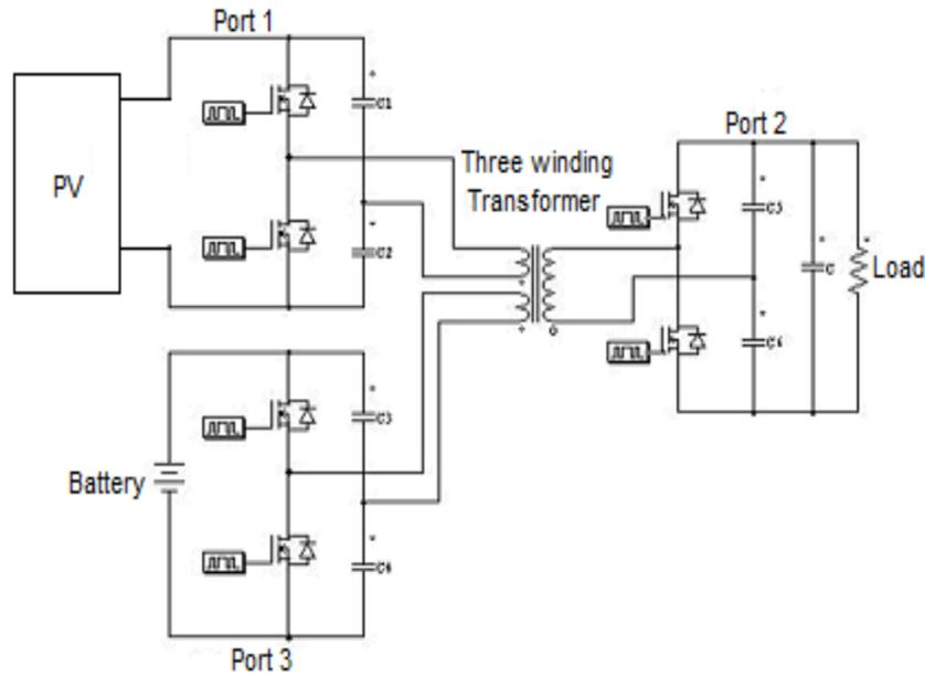
Figure 2-Three port half bridge converter
