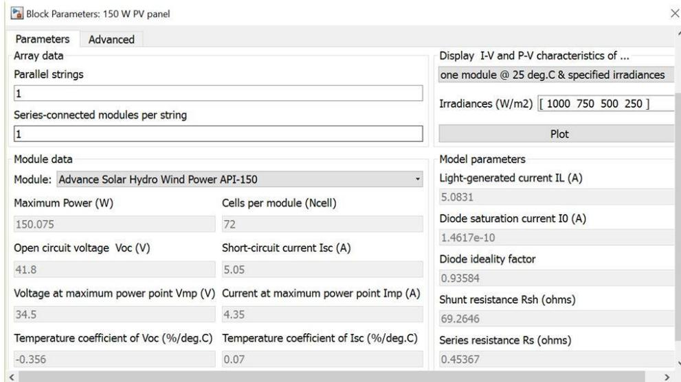
Figure 21-PV parameters utilized in Simulink
