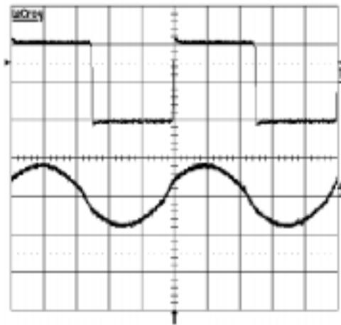
(b) Experimental results with Voltage (Top) 200V/div and current (Bottom) with 5A/div [2]
