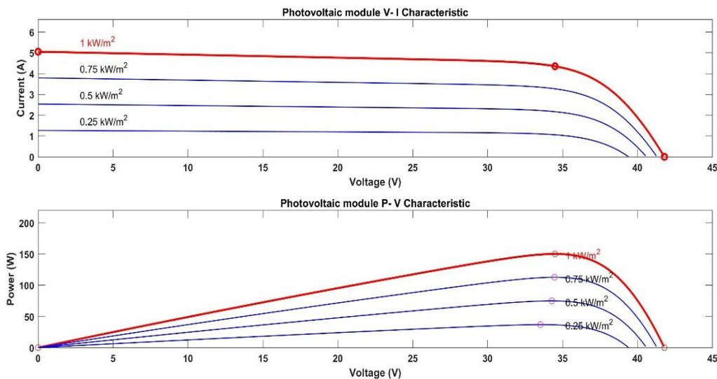
Figure 22-PV and IV curves for the PV cells assumed in the model
