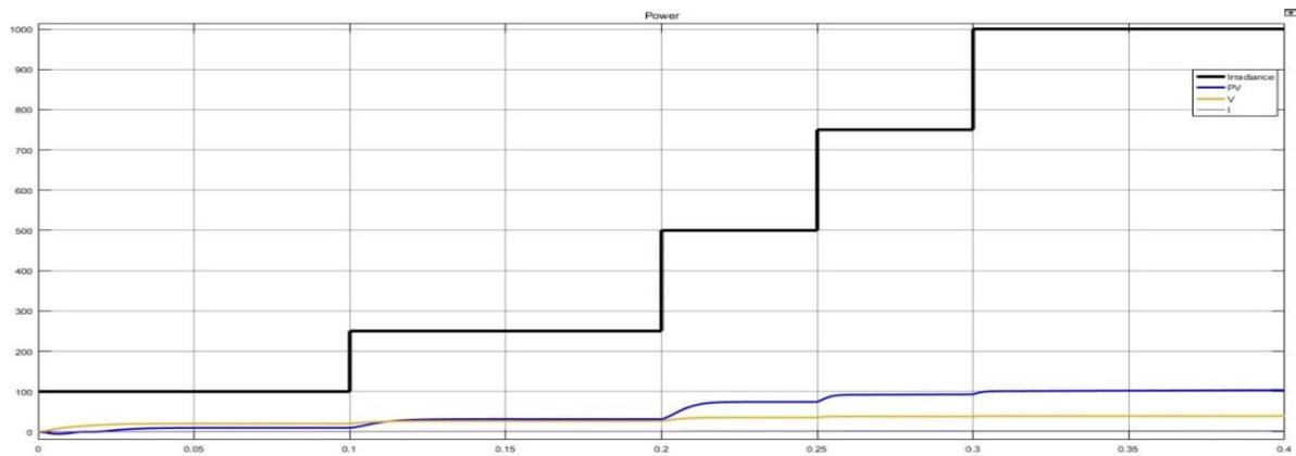
Figure 28-The effect of irradiance on PV power, voltage and current
