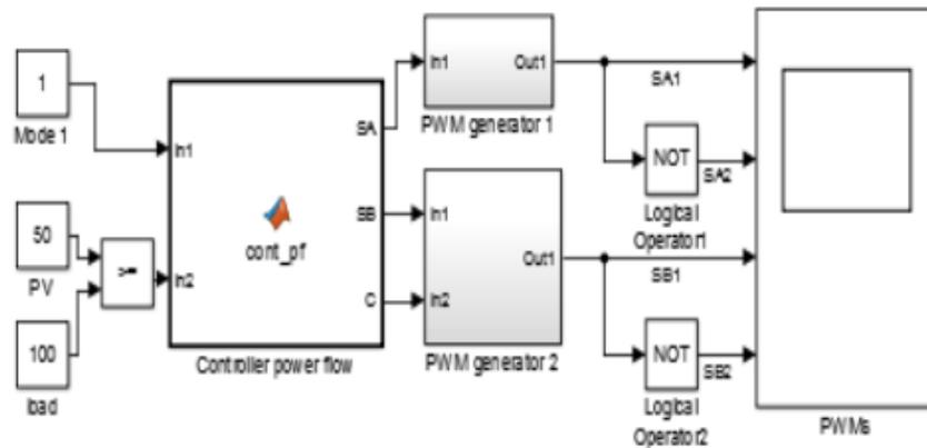
Figure 31- Design of controller for PWM Generation
