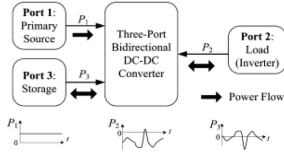
Figure 1-Energy flow in three port converters
