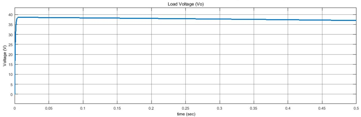
Figure 29-Output voltage at  $800 \text{ W/m}^2$
