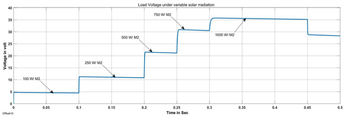
Figure 27-Output voltage for different irradiation cases
