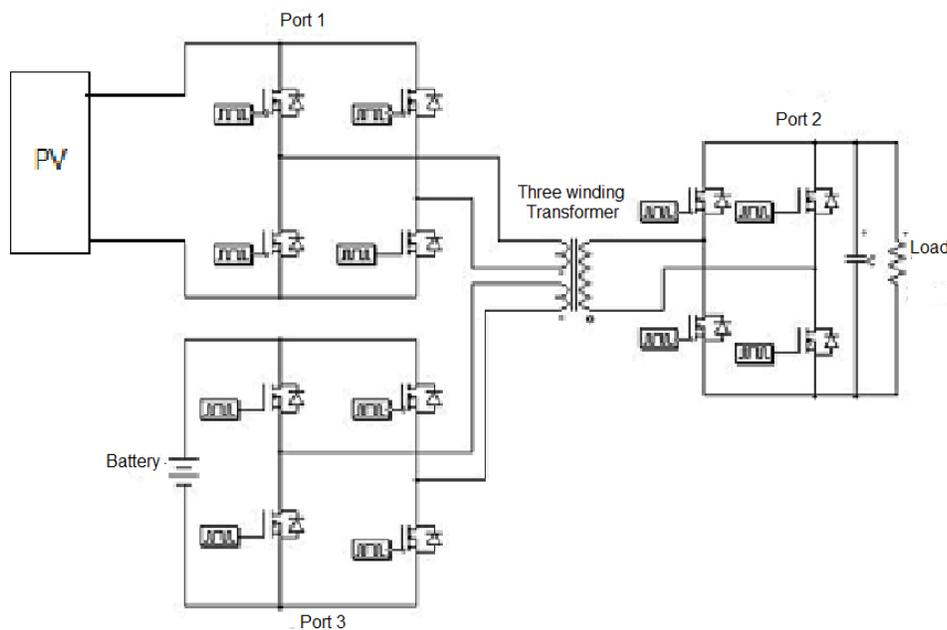
Figure 4- A three port full bridge converter
