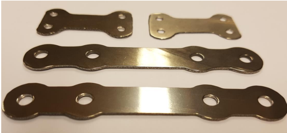
Figure 4.3 Photo of bone plates in the final form produced by Laser Melting Deposition (LMD) and mechanically processed for dimensions and roughness requirements [120].
