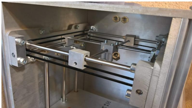
**Fig. 7.18.** Horizontal axes of the 3D printer.
