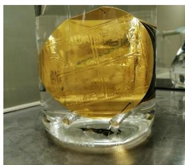
Fig. 9.26. Wafer immersion in the lift-off solution
