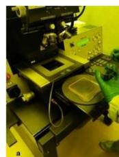
Fig. 7.15. a) orientation and b) fixing the wafer in the MA6 / BA6 equipment
