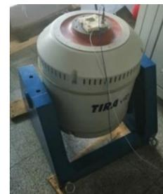
Fig. 9.64. Vibration testing of micro-electro-mechanical device
