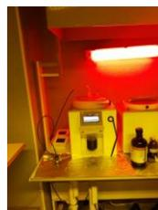
Fig. 7.9. Spinner Suss MicroTec equipment
