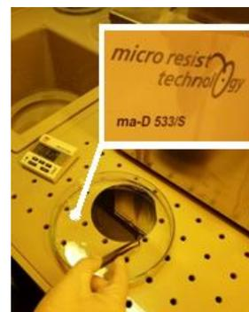
Fig. 9.25. Development with ma-D solution
