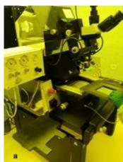
Fig. 7.14. a) orientation and b) fixing the mask in the MA6 / BA6 equipment
