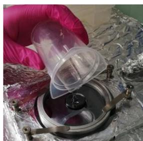
Fig. 7.42. Pouring the PDMS into the holder
