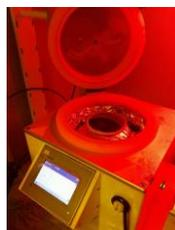
Fig. 7.8. LOR 10B photoresist deposited on the wafer
