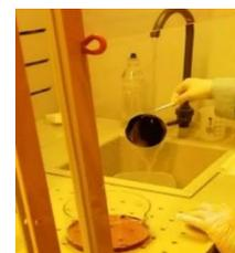
Fig. 7.17. Rinsing the wafer with deionized water
