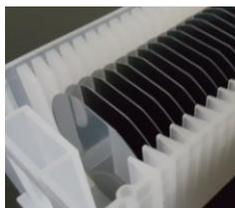
Fig. 2.3. Si wafers
