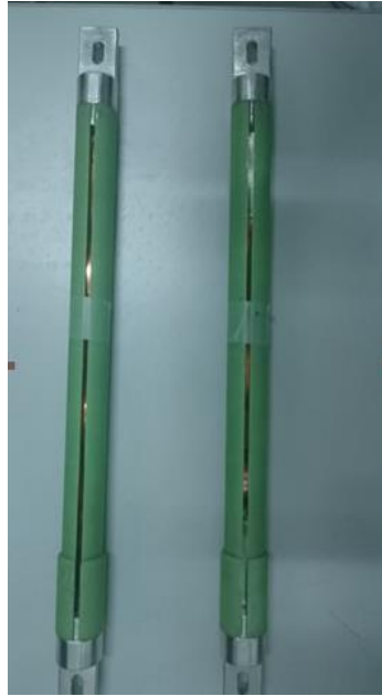
Fig. 6.15. HTS conductors assembled in housings.
