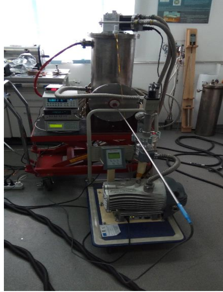
Fig. 7.8. EMSD assembly and magnetic field measurement system.
