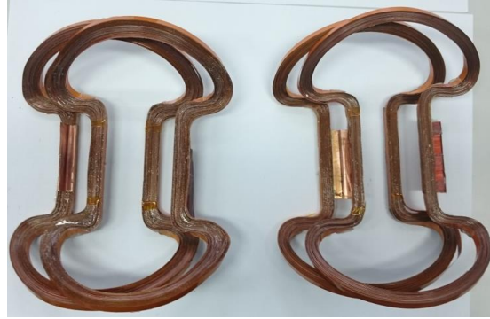
Fig. 6.2. HTS superconducting coils of the "saddle" type.
