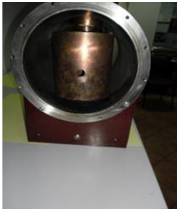
c. Cryostat - coils - thermal shield assembly, mounted in cryostat.
