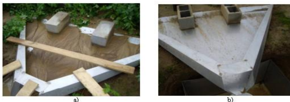
Fig. 2.9. Highlighting the erosion phenomenon in the case of non-partitioned furrows (a) and in the case of partitioned furrows (b) [102]
