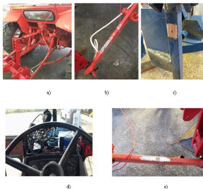
Fig. 4.52. Preparation of equipment for determining energy indices
