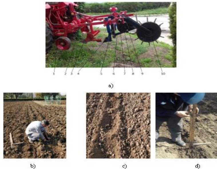
Fig. 4.58. Equipment fitted with the cam-tappet system a): 1 - copy wheel, 2 - frame, 3 – plough body, 4 - arrow blade, 5 - tappet holder, 6 - tappet, 7 - cam, 8 - chain wheel, 9 - chain, 10 - spur wheel) and aspects during the determination of qualitative indices b), c), d)
