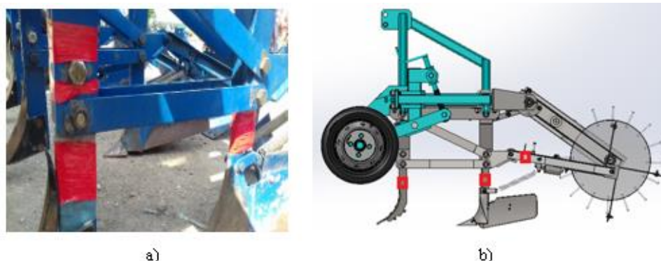
Fig. 4.26. Areas where the strain gages were mounted on DMBC-5 equipment (marked in red)
