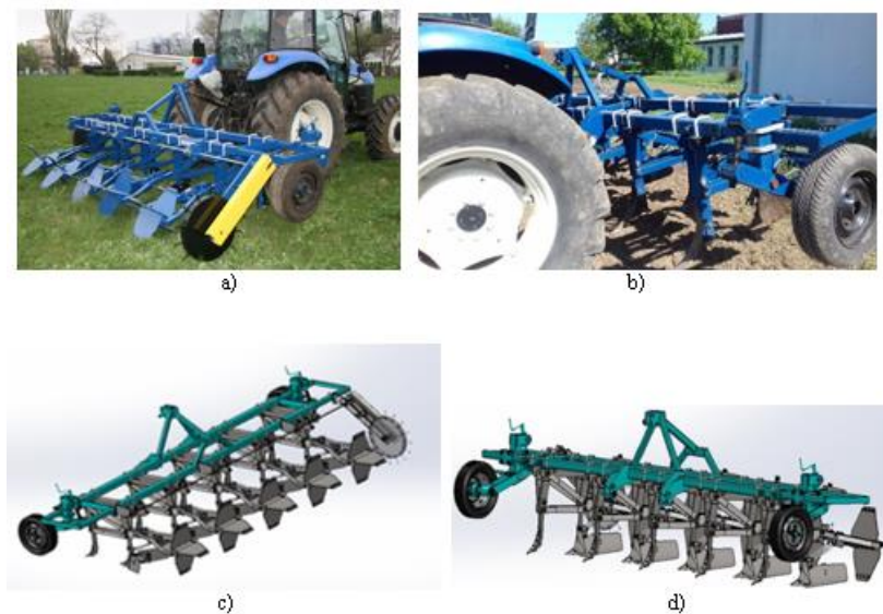
Fig. 2.40. DMBC-5 equipment for modelling the soil in partitioned furrows for weeding crops (a), (b), (c), (d) [106,108]
