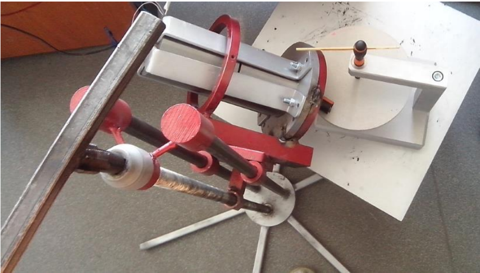
Fig. 5.4. Positioning system of the magnetostrictive actuator, general view.
