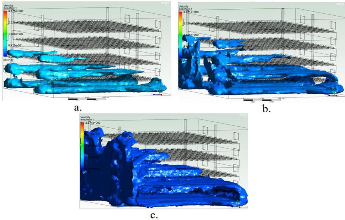
Fig. 4.14. Air speed distribution in the points where it reaches 0.6 m/s: a) fan working at 50 Hz simulation; b) fan working at 60 Hz simulation; c- fan working at 70 Hz simulation
