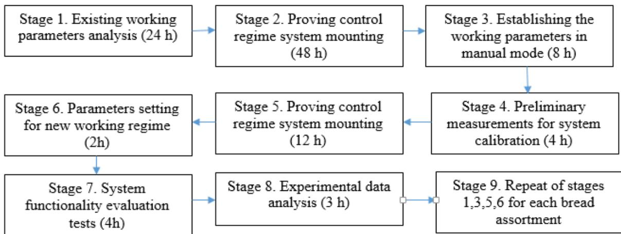
Fig. 5.33. The stages of implementing the control installation of the parameters of the proving work regime
