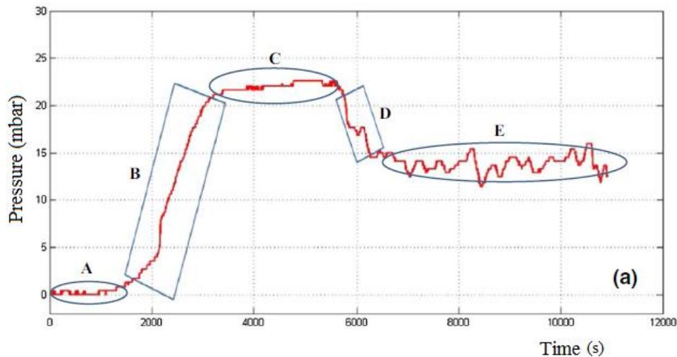
Fig. 3.36. Pressure variation during dough proving: A. lag period; B. development time (gas production); C) stability period; D) falling period (gas loss)
