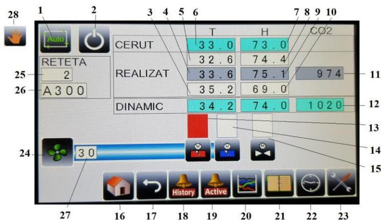
Fig. 5.29. Dynamic dough fermentation control plant control screen
