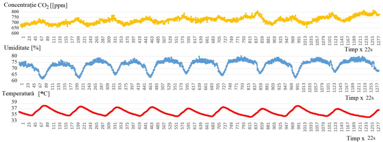
Fig. 5.60. Control of temperature and humidity, depending on the CO<sub>2</sub> concentration for Tibiletti prover
