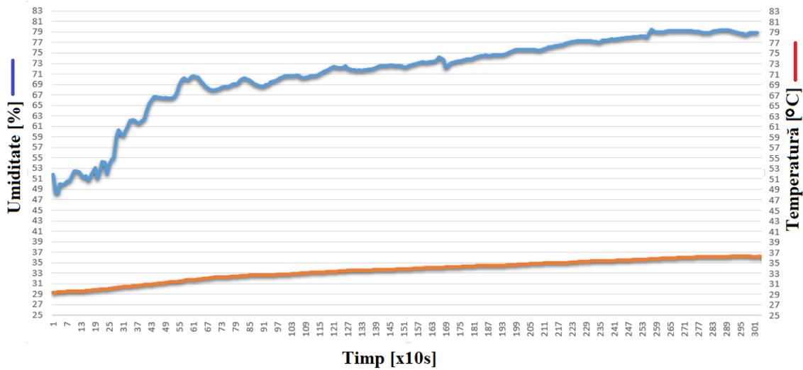
Fig. 5.53. Variation of temperature and humidity inside the prover during the fermentation process, when operating with conventional air conditioning, [74]
