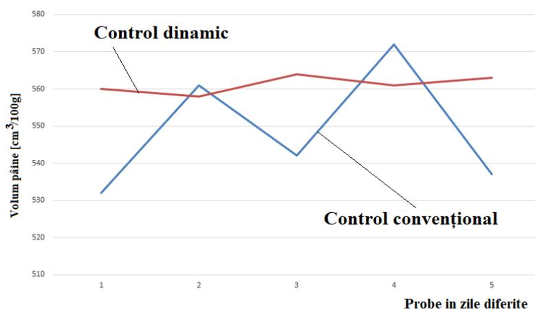
Fig. 5.60. Comparative analysis between the volume of breads obtained with dynamic air conditioning control versus conventional air conditioning control
