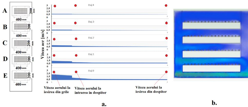
Fig. 5.71. Graphical representation of air velocity values measured on each floor of the leavener, using air distribution through equal grids
