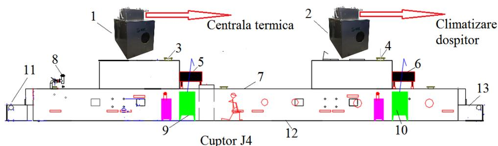
Fig. 4.3. Energy recovery systems mounted on J4 oven
