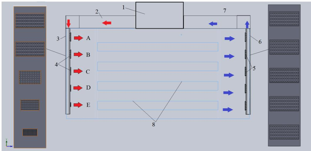
Fig. 4.10. The air distribution system design: 1-air conditioning system; 2-exterior pipes for air discharge; 3-interior pipes for air discharge; 4-air discharge grids; 5-air charge grids; 6-interior pipes for air charge; 7-exterior pipes for air charge; 8-prover floors
