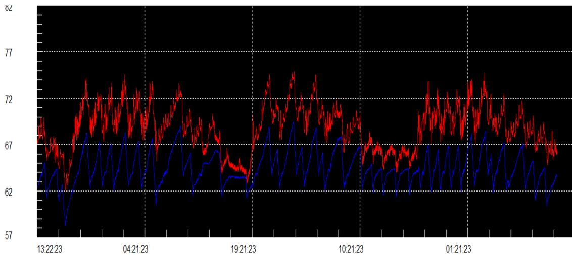
Fig. 5.78. Water temperature at the entrance to the recovery system (blue color), respectively at the exit of the recovery system (red color), measured for 3 days
