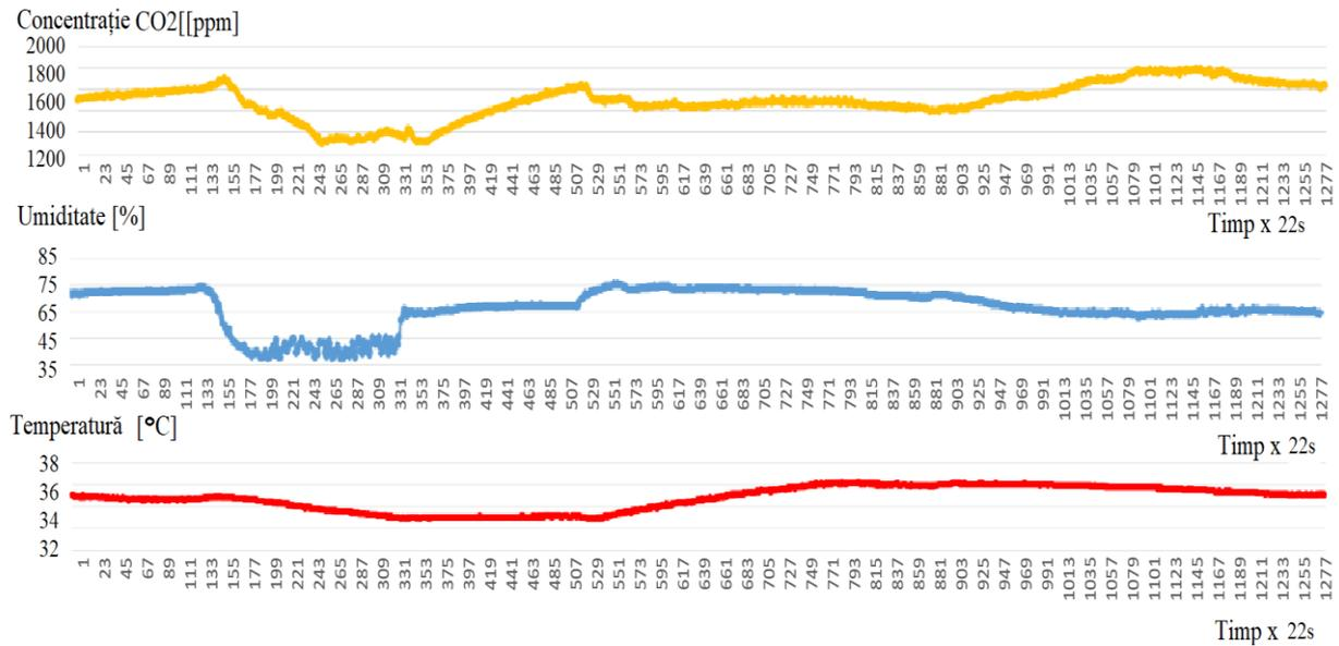
Fig. 5.63. Automatic control of temperature and humidity according to the CO<sub>2</sub> value released in the spiral prover, Tecnpool
