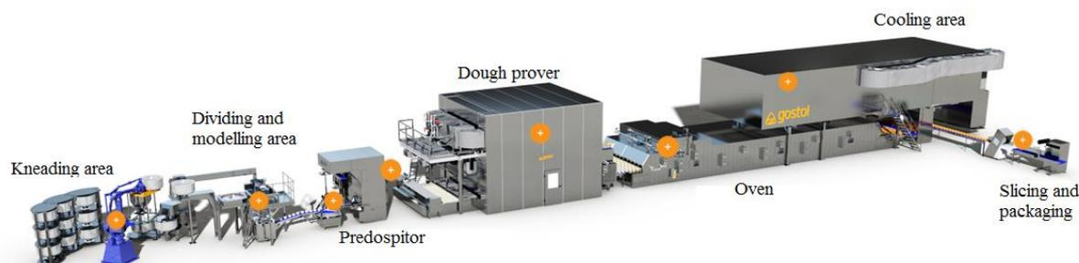
Fig. 2.2. Modern technological line for bread making with tank dough fermentation
