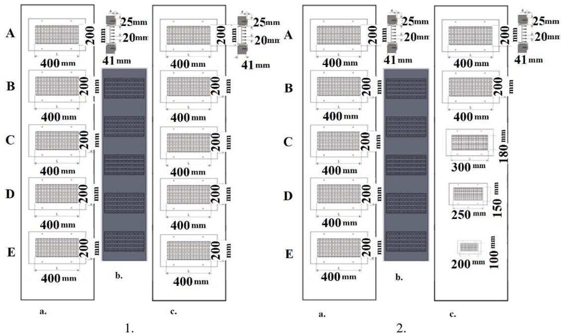
Fig. 4.13. 1.First case – a) Interior charge grids, b) Interior discharge grids designed in Solid Works, c) Interior discharge grids; 2. Second case – a). Interior charge grids, b) Interior discharge grids designed in Solid Works; c) Interior discharge grids
