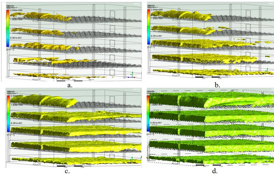
Fig. 4.17. Air speed distribution in all points where it reaches 0.6 m/s: a) simulation with fan functioning at 20 Hz; b) simulation with fan functioning at 30 Hz; c) simulation with fan functioning at 40 Hz; d) simulation with fan functioning at 50 Hz
