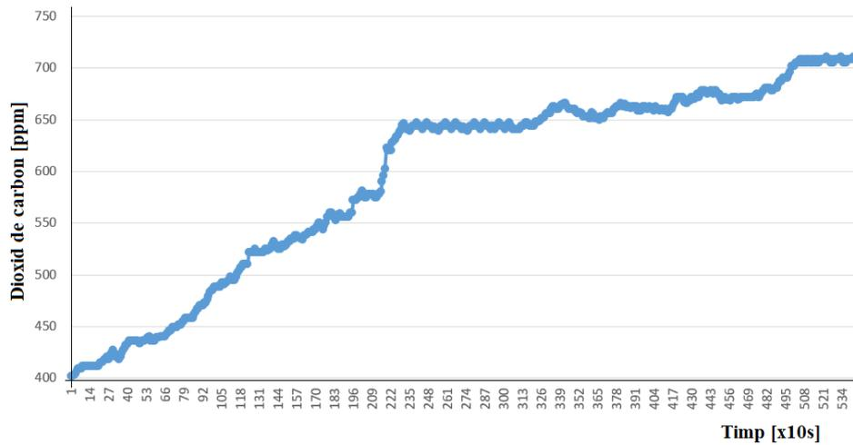
Fig. 5.46. Variation of carbon dioxide released for the first 90 minutes of Werner prover working with system set in manual mode
