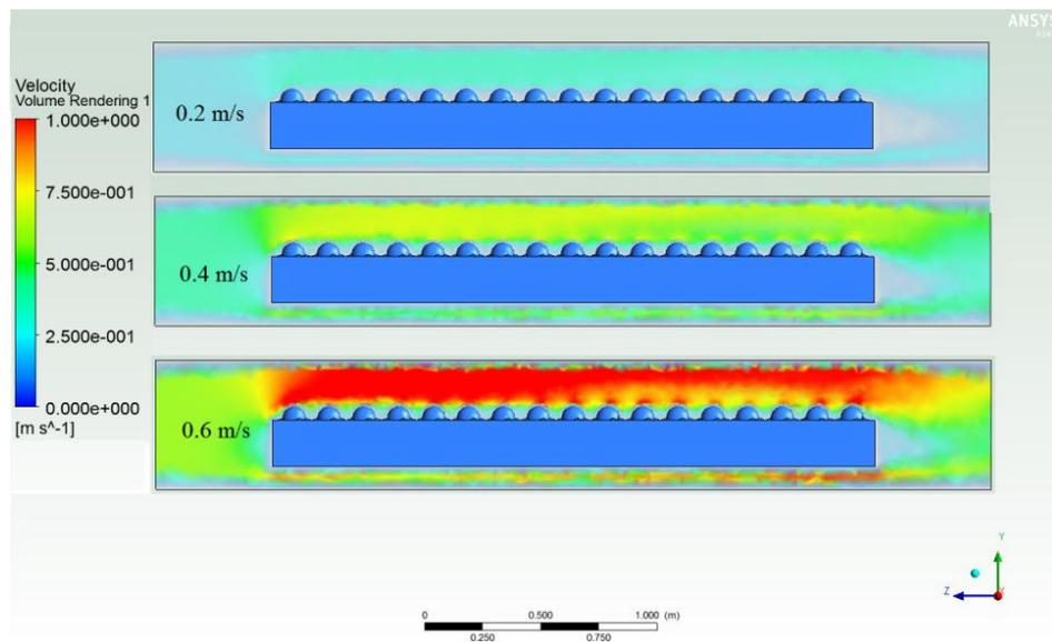
Fig. 4.11. Air speed distribution in the proving chamber based on the air speed
