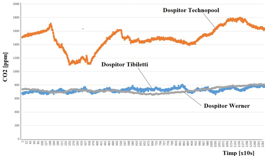
Fig. 5.64. Carbon dioxide concentrations recorded in the 3 provers for 4 hours
