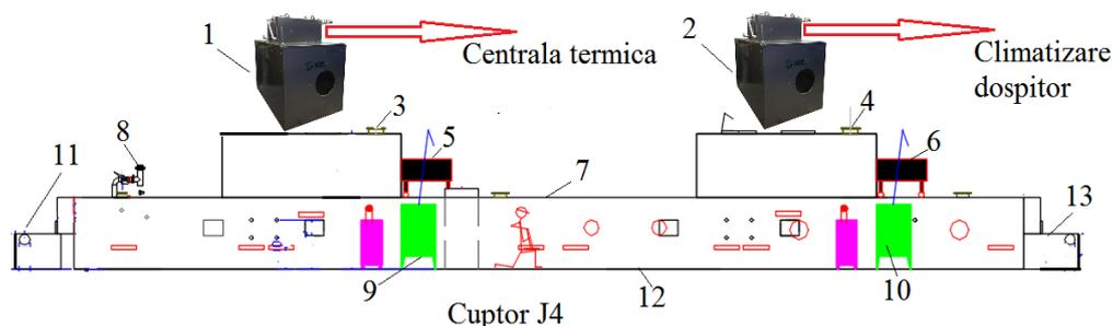
Fig. 4.3. Energy recovery systems mounted on J4 oven
