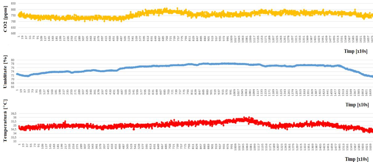
Fig. 5.55. Variation of temperature, humidity and concentration of carbon dioxide in the operation of the leavener with the dynamically controlled air conditioning system, [74]
