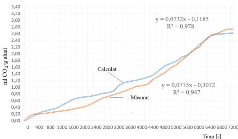
Fig. 5.74. Checking the mathematical model after the compressibility factor Z has been introduced to the FA<sub>1</sub>-650 flour, [73]
