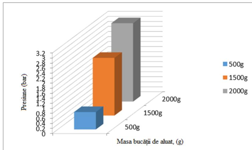
Fig. 5.36. Pressure in the experimental chamber for different amounts of dough
