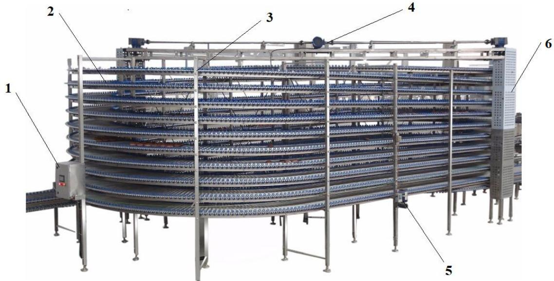
Fig. 5.12. Spiral-type prover, Tecnopool, [183]
