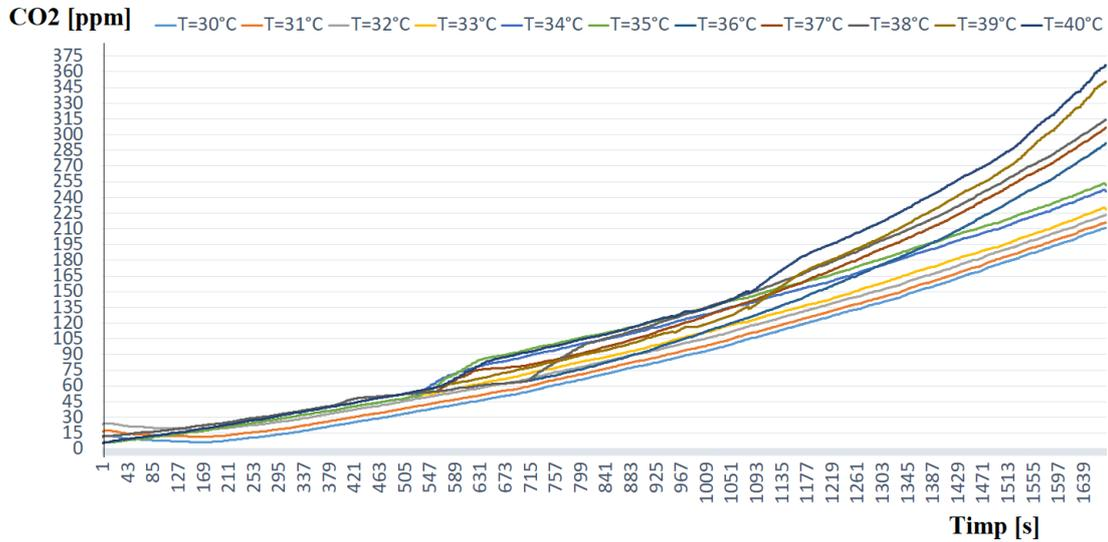
Fig. 5.41. CO<sub>2</sub> values recorded during the leavening process for a piece of dough at 11 different temperatures (from grade to grade), [72]
