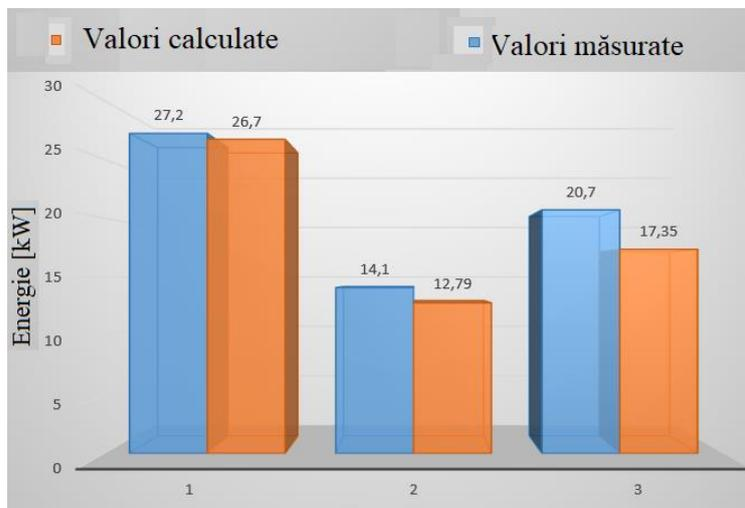
Fig. 5.73. Energy consumption measured, respectively calculated for the air conditioner of the leavener, in the 3 operating modes, [71]
