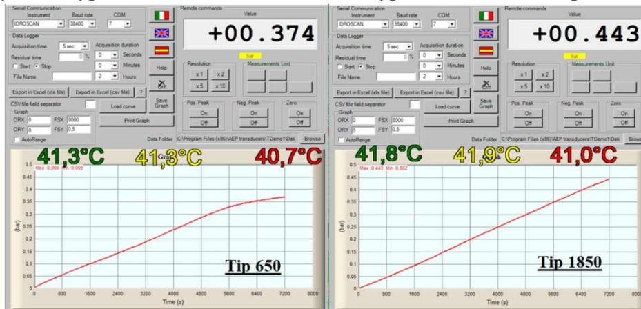
Fig. 5.39. Reactor pressure when using different extraction flours: left type 650; right-type 1850 (ash content)
