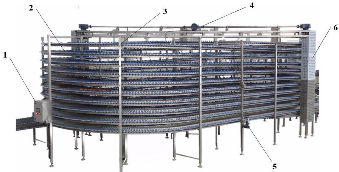
Fig. 5.12. Spiral-type prover, Tecnopool, [183]
