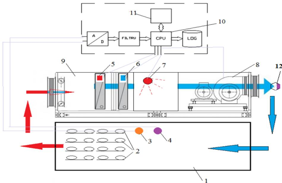
Fig. 5.18. Components of the air conditioning system for the control of the concentration of carbon dioxide in provers, [74]
