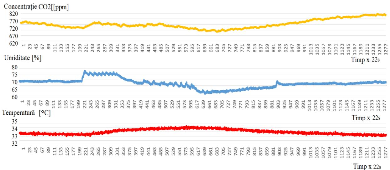
Fig. 5.61. Automatic control of temperature and humidity according to the value of CO<sub>2</sub> released by the prover of the Werner line
