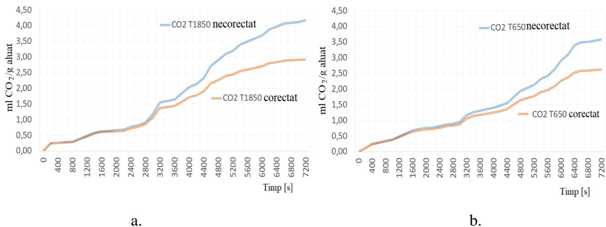
Fig. 4.19. Comparative analysis of the volumes of carbon dioxide calculated when using FA1-650 and FI-1850 flours, respectively, in the fermentation process at 40 ° C, with and without the introduction of the compressibility factor,  $Z$ , [73]
