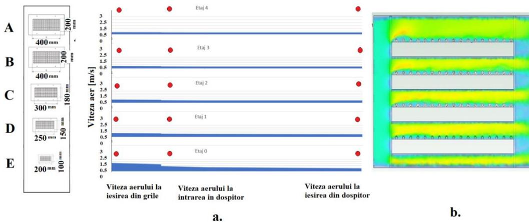
Fig. 5.72. Graphical representation of air velocity values measured on each floor of the leavener, using the distribution of recirculated air through grids of different sizes
