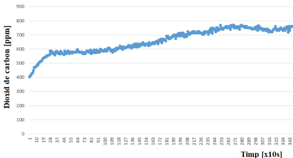
Fig. 5.48. The CO<sub>2</sub> variation for the first 60 minutes of working with the Tibiletti prover, in manual mode
