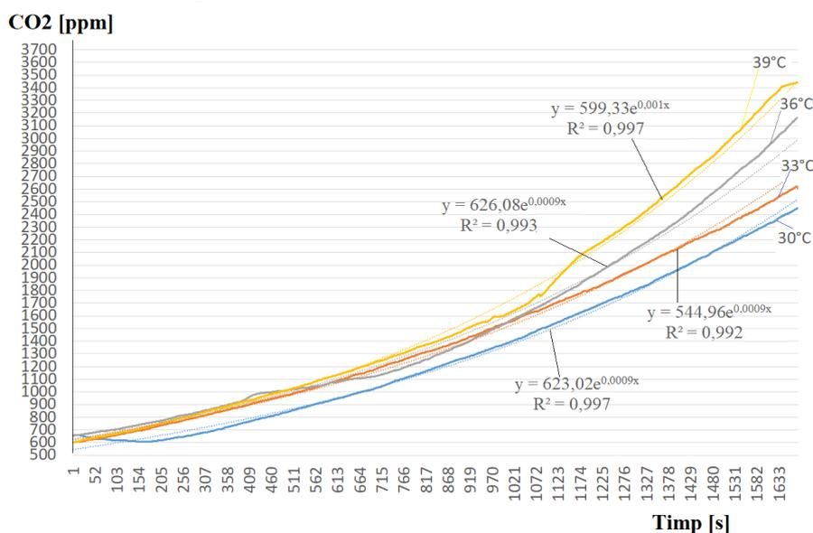
Fig. 5.44. The variation of CO<sub>2</sub> released for the nine pieces of dough proving at 4 different temperatures, [72]
