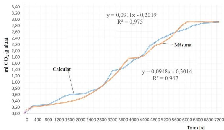
Fig. 5.75. Checking the mathematical model after the compressibility factor  $Z$  was introduced to the FI-1850 flour, [73]
