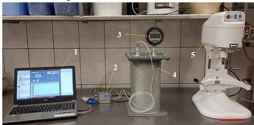
Fig. 5.9. Experimental stand for the fermentation process study of dough
