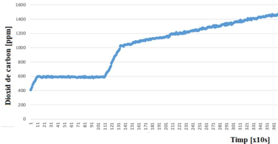
Fig. 5.50. Variation of carbon dioxide concentration for the first 60 minutes of operating with the Tecnopool prover in manual mode
