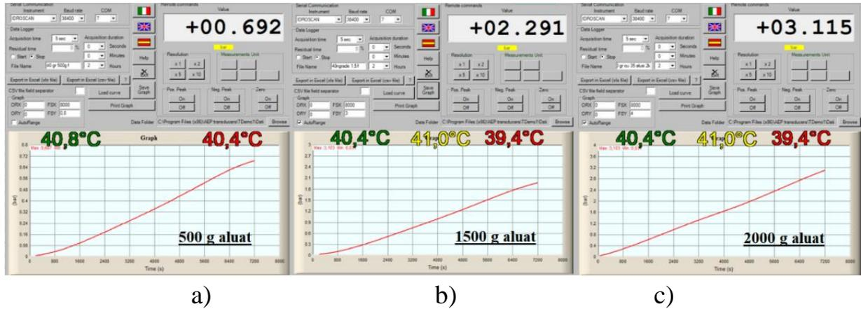
Fig. 5.35. Variation of pressure in the reactor for three different amounts of dough
