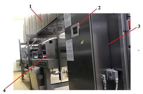
Fig.5.15. Werner Pfleiderer plate prover, [215] 1. proving chamber; 2. touch screen for viewing the prover's parameters; 3. control panel; 4. shaper for long dough
