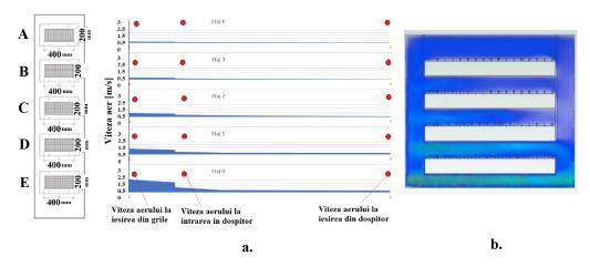
Fig. 5.71. Graphical representation of air velocity values measured on each floor of the leavener, using air distribution through equal grids
