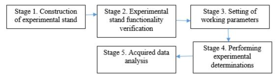
Fig. 5.8. The steps of obtaining experimental data using the experimental stand
