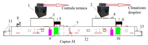
Fig. 4.3. Energy recovery systems mounted on J4 oven 1. gas-water recovery system in first baking area; 2. gas-water recovery system in second baking area; 3. area 1 burnt gases evacuation tunnel; 4. area 2 burnt gases evacuation tunnel; 5. area 1 pellets burner; 6. area 2 pellets burner; 7. operator; 8. steam intake; 9,10. Area 1 and 2 pellets reserves
