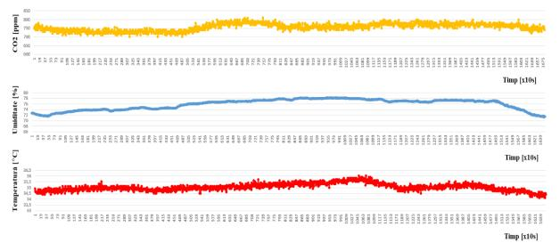
Fig. 5.55. Variation of temperature, humidity and concentration of carbon dioxide in the operation of the leavener with the dynamically controlled air conditioning system, [74]
