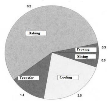
Fig. 1.12. Dough piece lossess during processing (%), [24]
