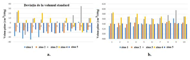
Fig. 5.56. Variation of the volume of breads obtained for the leavener with conventional air conditioning
