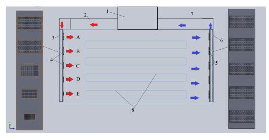
Fig. 4.10. The air distribution system design: 1-air conditioning system; 2-exterior pipes for air discharge; 3-interior pipes for air discharge; 4-air discharge grids; 5-air charge grids; 6-interior pipes for air charge; 7-exterior pipes for air charge; 8-prover floors
