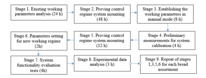
Fig. 5.33. The stages of implementing the control installation of the parameters of the proving work regime
