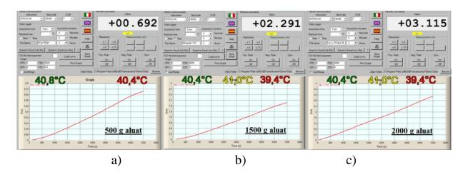
Fig. 5.35. Variation of pressure in the reactor for three different amounts of dough a-500 g dough 5s; b-1500 g dough; c-2000 g dough
