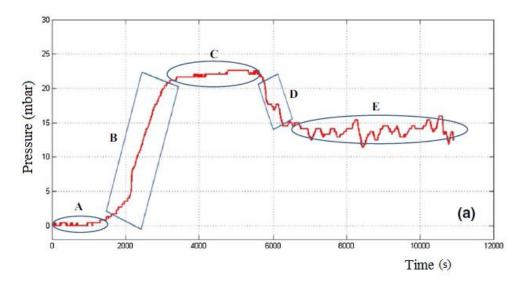
Fig. 3.36. Pressure variation during dough proving: A. lag period; B. development time (gas production); C) stability period; D) falling period (gas loss)
