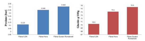
Fig. 5.38. The pressure in the reactor and varying the amount of sugar to flour FA-650 from different mills
