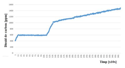
Fig. 5.50. Variation of carbon dioxide concentration for the first 60 minutes of operating with the Tecnopool prover in manual mode
