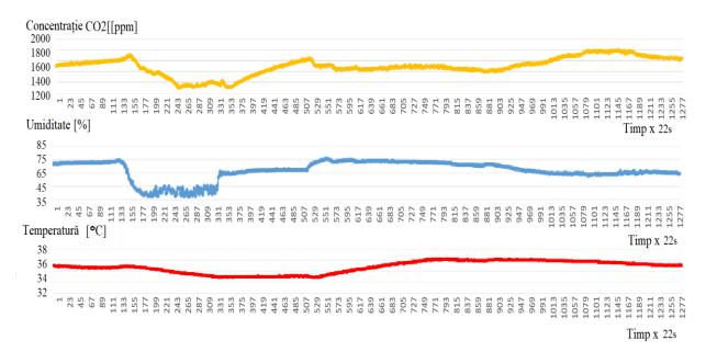
Fig. 5.63. Automatic control of temperature and humidity according to the CO<sub>2</sub> value released in the spiral prover, Tecnopool
