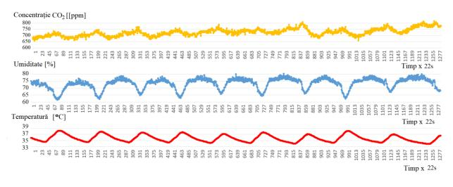
Fig. 5.60. Control of temperature and humidity, depending on the CO<sub>2</sub> concentration for Tibiletti prover
