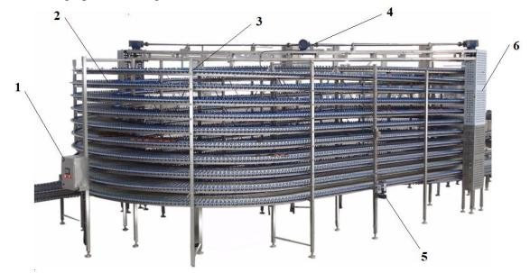
Fig. 5.12. Spiral-type prover, Tecnopool, [183]1. control panel; 2. conveyor belt; 3. frame; 4. horizontal transmission; 5. belt chain lubrication system; 6. vertical transmission
