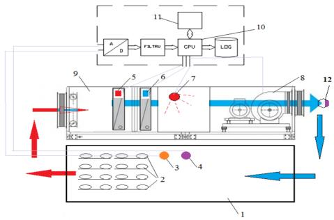
Fig. 5.18. Components of the air conditioning system for the control of the concentration of carbon dioxide in provers, [74]
