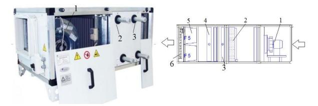
Fig. 2.32. Air conditioning unit for dough prover, [213] ventilator; 2. drainer; 3. heat exchanger with cold water; 4. heat exchanger with hot water; 5. hepa filter; 6. grid flap
