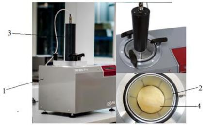
Fig. 3.5. Chopin rheofermentometer, [196] 1-device; 2-fermentation chamber; 3-piston body; 4-dough piece
