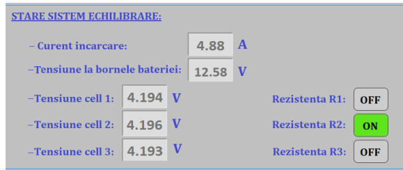
Fig. 5.21. Balancing system status - signaling resistance status balancing cell 2
