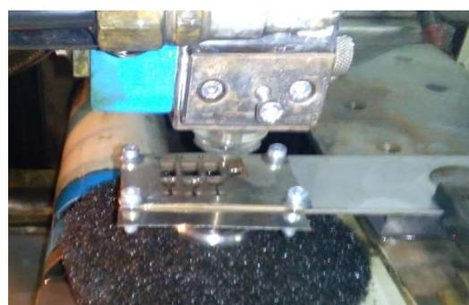
**Figure 5.18.** Cutting test structures using wire EDM
