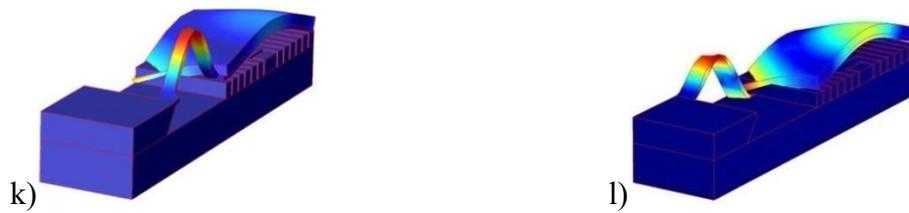
**Figure 2.4** Deformations for the first six eigenstructural modes. The results for the left column (console with a central beam) are scaled by 2.5 and for the right column (console with two side beams) by 2.
