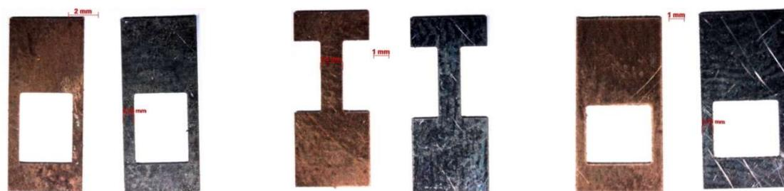
12mm x5mm, 0,75mm beams    12mm x5mm, 1,5mm beam    12mm x 6mm, 0,75mm beams
