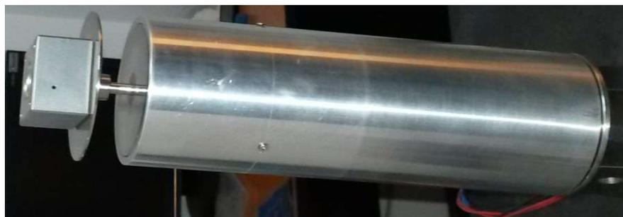
**Figure 5.12** Magnetostrictive linear actuator - practical realization
