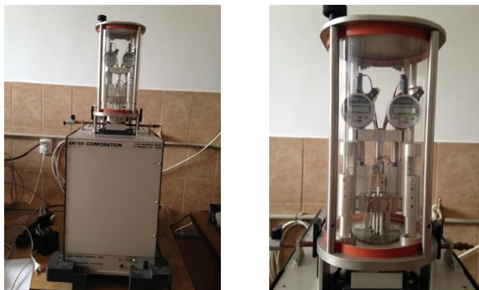
Figura 5.9. Dilatometrul termic vertical, model Unitherm 1161V
