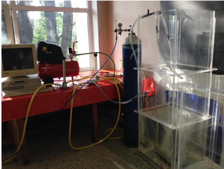
Fig. 6.2. Overview of the experimental installation to the introduction of a mixture of gases (atmospheric air and oxygen)
