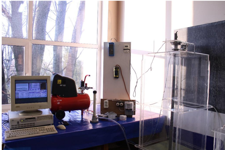
Fig. 6.1. Overview of the experimental installation for blowing atmospheric air
