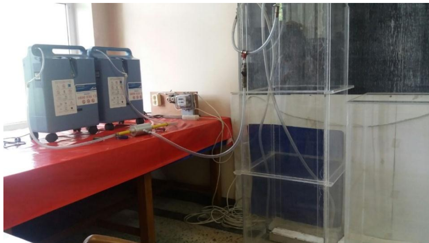
Fig. 6.3. Overview of the experimental installation for the introduction of air with low nitrogen content
