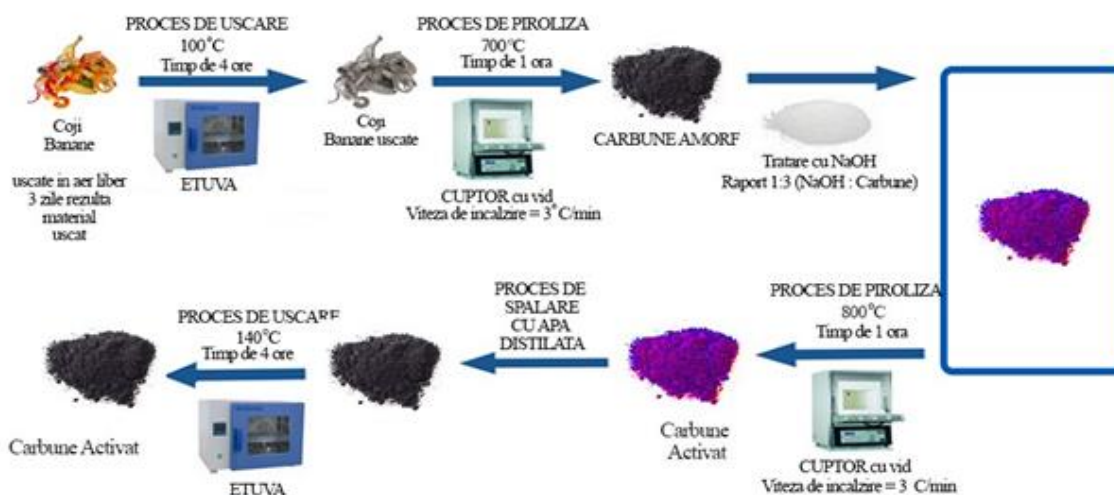
Figure 7 – The process of obtaining activated charcoal from banana peels – CBvid
