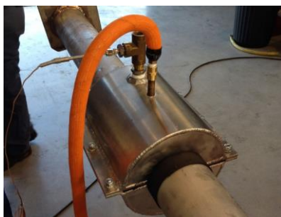
Fig. 1.1 - Rigid freezing device with liquid nitrogen circulation
