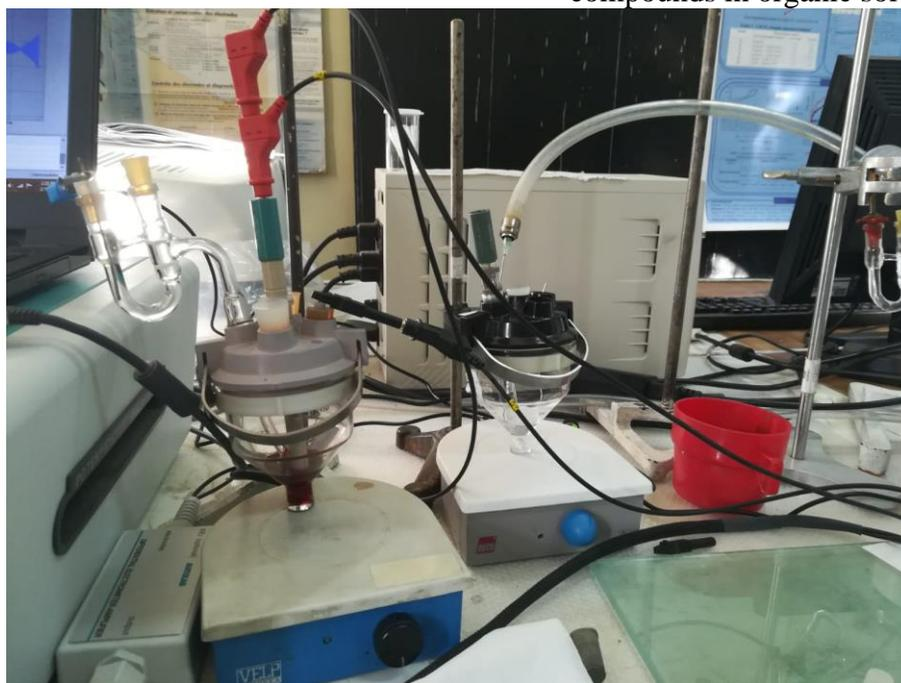
**Fig. 4.3.** Cells for the preparation of CMEs by electrolysis at controlled potential (left) and for their conditioning (right)
