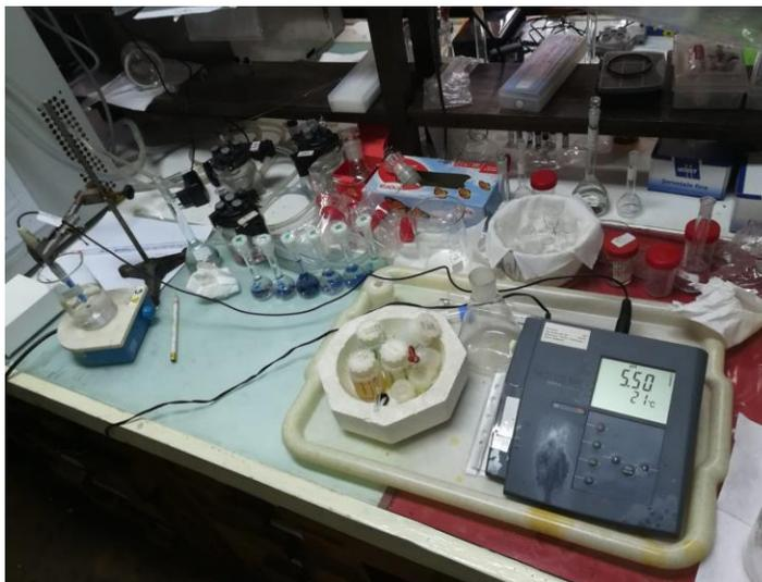
**Fig. 4.5.** Installation for measuring the pH of the electrolyte used in the conditioning cell for CMEs
