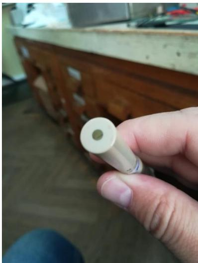
**Fig. 4.4.** CPE modified glassy carbon electrode
