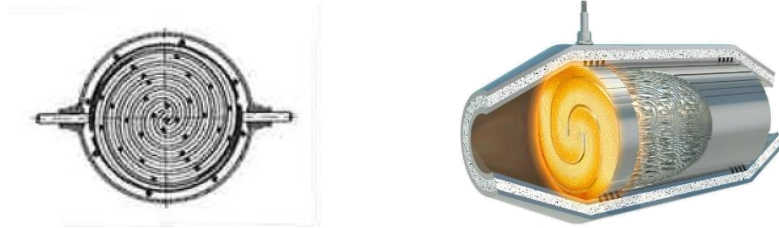
Figure 6 Emitec EHC build cross-section [3.2] and cut-out [3.1]
