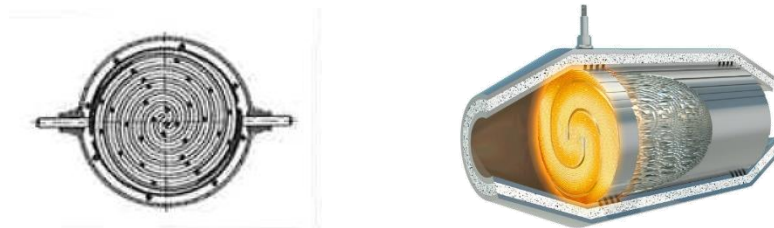
Figure 6 Emitec EHC build cross-section [3.2] and cut-out [3.1]
