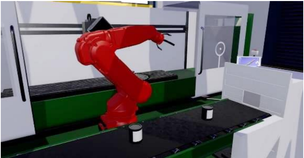
Figure 10. Machining center serviced by an articulated arm industrial robot
