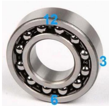
FIG. 13. Placement of faults relative to the loading area (6), opposite the loading area (12) and orthogonal to it (3).
