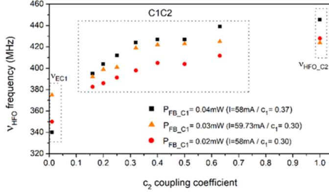
**Figure 4.5**  $v_{HFO}$  frequency behavior function of  $c_2$  coupling coefficient of C2 cavity for three C1 cavity feedback powers ( $P_{FB\_C1}$ )
