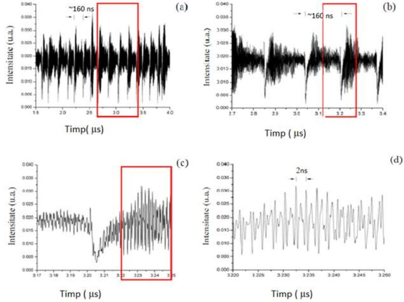
**Figure 2.10** The intensity time series: (a) LFF chaotic dynamic; (b) detail of the area marked in (a); (c) rapid oscillations - detail on the area marked in (b); (d) rapid oscillations - detail on the area marked in (c). Operating parameters:  $I = 1.04 \times I_{th}$ ,  $t = 24^\circ C$  and  $L_{ext} = 30cm$ . In (a) - (b) and (c) the characteristic average periods of the LFF oscillations and of the oscillations of the external cavity modes are indicated.
