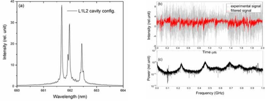
**Figure 6.1** D-ECSL system emission characteristics; (a) optical spectrum, (b) power intensity time series and (c) associated power spectrum for  $I= 58$  mA,  $t= 24.9$  °C,  $c_1= 1.0$  și  $c_2=0.72$ .
