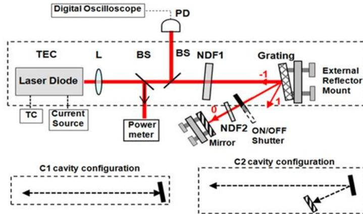
**Figure 4.1** Scheme of D-ECSL experimental setup. TEC, thermo-electric controller mount; TC, temperature controller; L, collimation lens system; BS, beam splitters; NDF 1, neutral continuously variable density filter; NDF 2, neutral step-variable density filter; PD, photodetector; -1, 0, 1 - diffraction orders.
