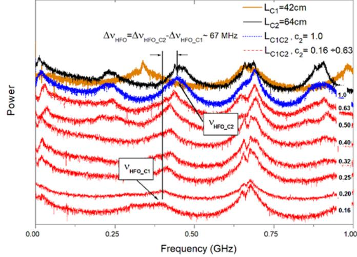
**Figure 4.4**  $\nu_{HFO}$  frequency shift with C2 feedback variation. Power spectra for C1, C2 and C1C2 ( $c_2 = 1.0$ ) cavity configurations are the same as in Figure 2. Parameters:  $I_{th}$  threshold current,  $c_1 = 0.37$ , and  $t = 24.9^\circ\text{C}$
