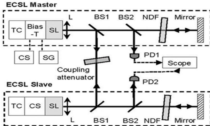
**Figure 5.1** Setup of two chaotic lasers bidirectionally coupled into a master-slave synchronization scheme. Master laser is driven by a periodic signal generator (SG); SL-semiconductor laser; ECSL-external cavity semiconductor laser system; BS-beam-splitter; TC-temperature controller; CS- direct current source Bias-T-frequency multiplexor.
