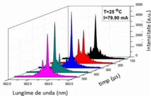
Figure 3.6 The effect of mode-hopping at 79.9 mA injection current and 24.9  $^{\circ}\text{C}$  diode temperature. Series of optical spectra of laser emission-free acquired at an interval of 100  $\mu\text{s}$
