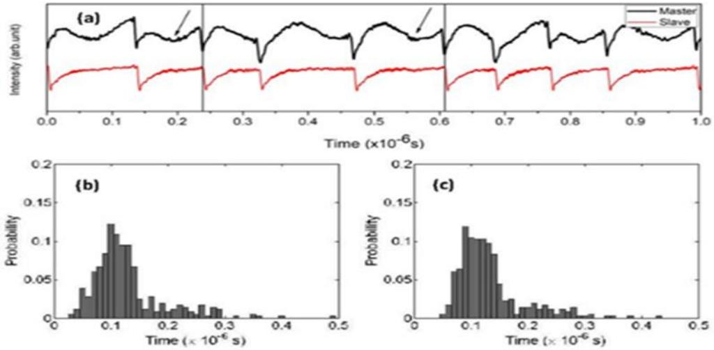
**Figure 5.5** Master and slave systems chaotically coupled at 8 MHz: (a) intensity time series for master and slave coupled systems; (b) and (c) histograms of power dropouts for master and slave, respectively. Arrows indicate intensity oscillations induced by the modulation for which master LFF dynamics does not engage
