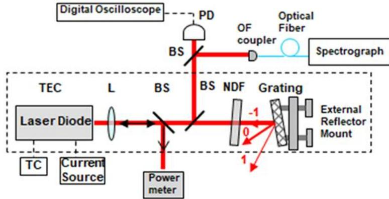
**Figure 3.1** The experimental setup. TEC, thermo-electric controller mount; TC, temperature controller; L, collimation lens systems; BS, beam splitters; NDF, neutral continuously variable density filter; PD, photodetector; OF, optical fiber; -1, 0, 1, diffraction orders.
