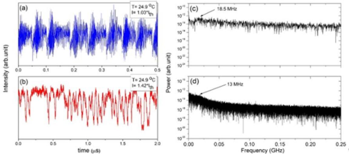
**Figure 3.8** The intensity time series and associated power spectra for the injection currents (a)/(c)  $I_1=1.03 \cdot I_{th}$  and (b)/(d)  $I = 1.42 \cdot I_{th}$ , when the mirror is used, and  $I_{th}=58 \text{ mA}$ ,  $t = 24.9^\circ\text{C}$ .
