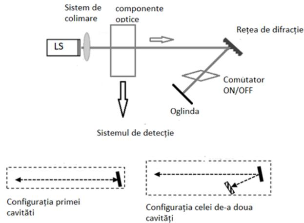
*Figure 2.15 Scheme of D-ECSL experimental setup*
