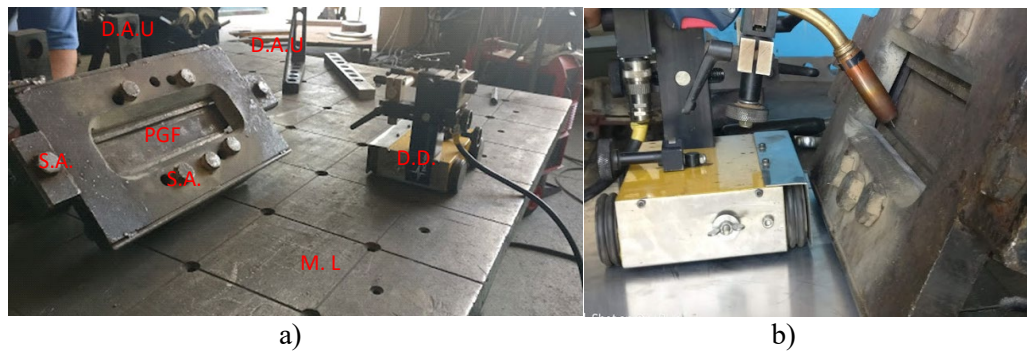
Fig. 6.40. Experimental stand - reconditioning through process FCAWm a) positioning sample into the device at 45 °, b) positioning torch welding SA - system assembly device, ML - work table, PGF – friction liner holder, DD - device displacement welding torch (for mechanization), SAD - devices for ensuring the angle of inclination
